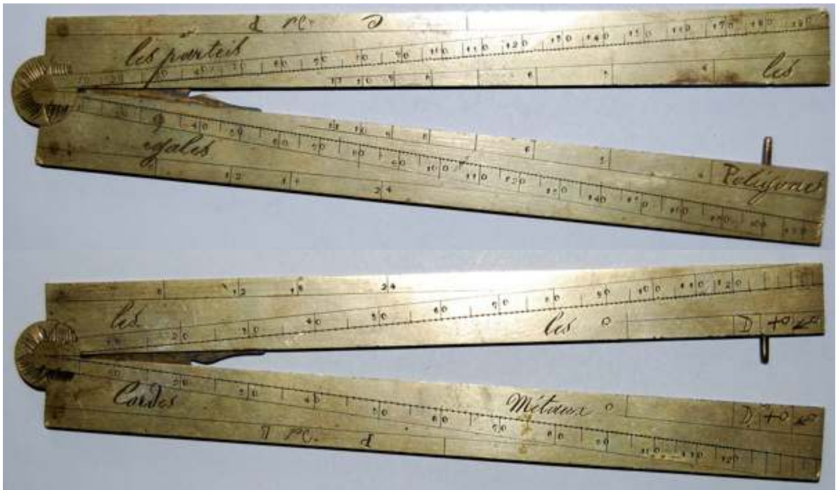
Fig. 173 French brass sector showing upper and lower faces
