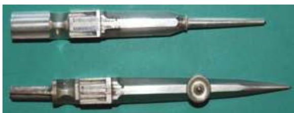
Fig. 6 Needle points showing socket and shank of slip joints
