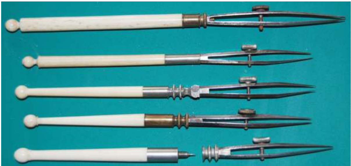
Fig. 171 French drawing pens - from the top: (a) bone handled pen from cheap brass set, (b) ivory handled fine line pen, finely turned finial, German silver ferrule, from a top quality set (c) lifting nib pen with ivory handle and pricker inside from the same set as 'b', (d) ivory handled pen from better quality brass set, (e) ivory handled pen with handle unscrewed to show pricker.
