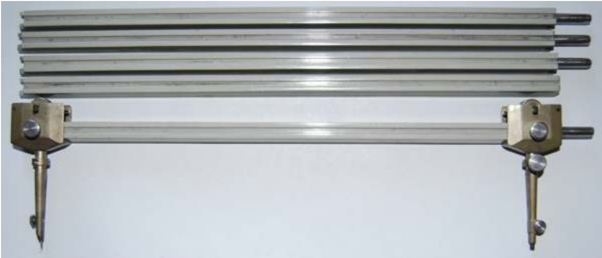
Fig. 120 Lee Guinness beam compass
