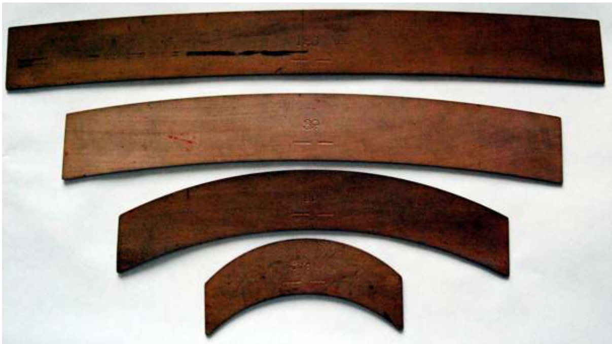
Fig. 78 Pear wood railway curves from a set of 50 by W F Stanley
