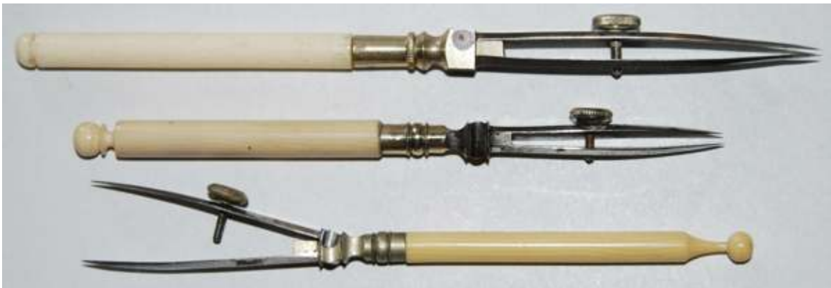
Fig. 185 German pens with lifting nibs.
