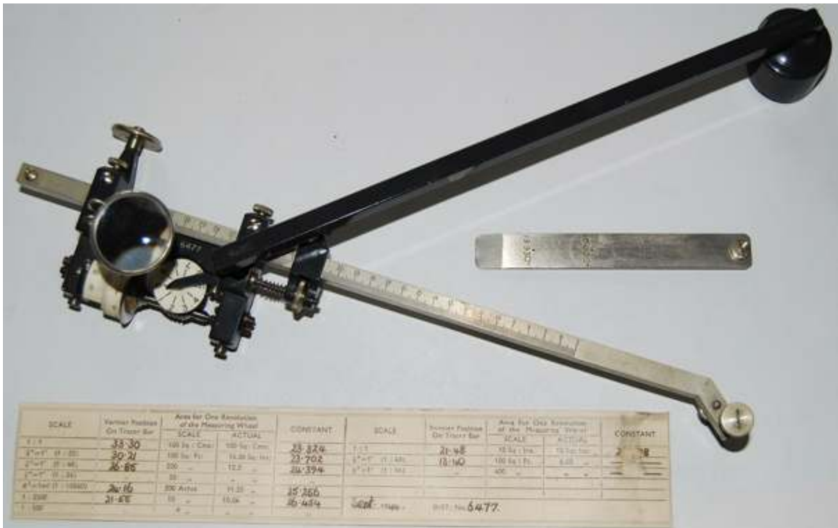
Fig. 142 Allbrit adjustable planimeter no. 6477, made in September 1944 by W F Stanley
