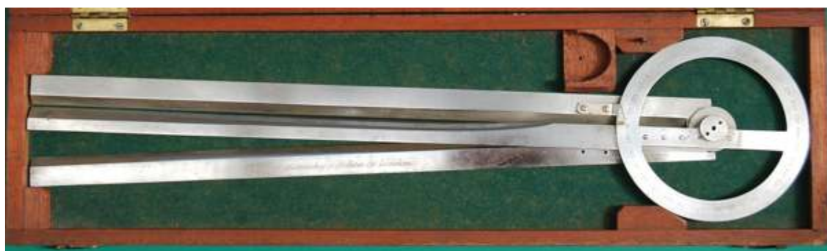
Fig. 156 Bottomly, 11 Billiter Street, London, station pointer, dating from the 1880s
