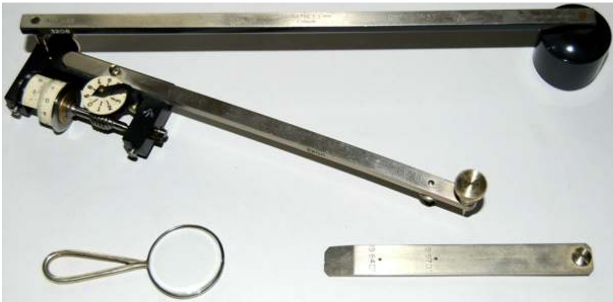
Fig. 143 W F Stanley 'Allbrit' fixed scale planimeter no. 3208 supplied to the War Office on 24th April 1937
