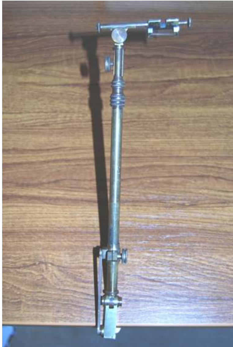
Figs. 324/5 Camera Lucida (Chambre Claire Universelle) made in France and imported by Lechertier Barbe Ltd., 95 Jermyn Street, St. James's, London SW1. It is made of brass and has eleven of its original twelve lenses remaining. Complete with instruction leaflet. Probably 1920s.
