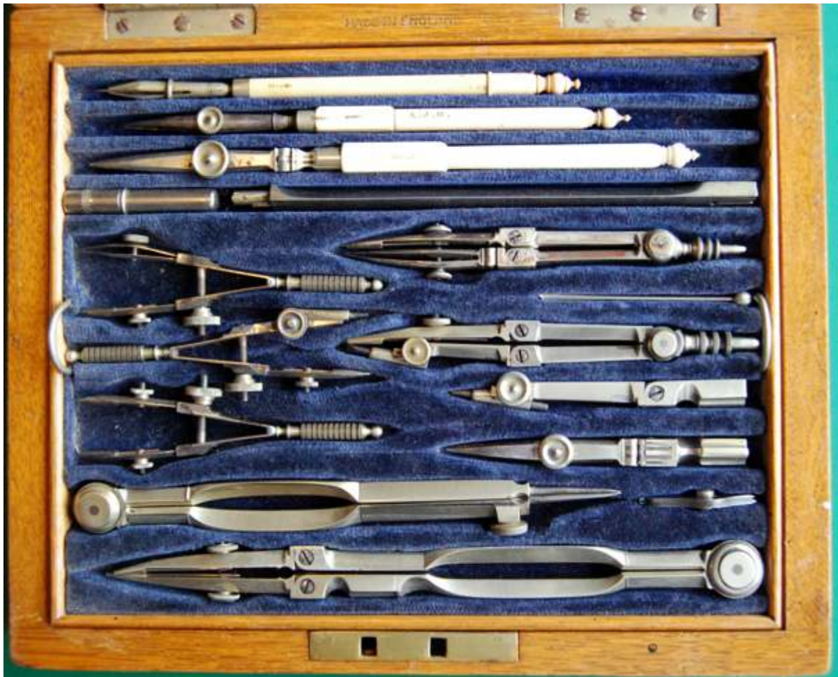
Fig. 3 W F Stanley oak-cased set of electrum instruments
