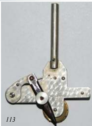
Figs. 112 to 114 Beam compass by unknown maker
