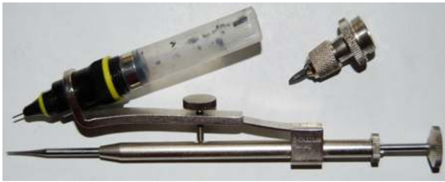
Fig. 236 Staedtler Mars Superbow with Rotring Variant pen attached
