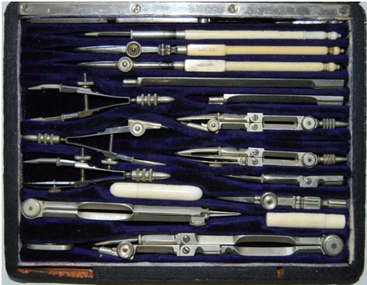
Fig. 260 W H Harling, 47 Finsbury Pavement, full set of small size (4 1/2 inch) drawing instruments with screw off needle points, late 19th century. A top quality set in a Russian leather case.
