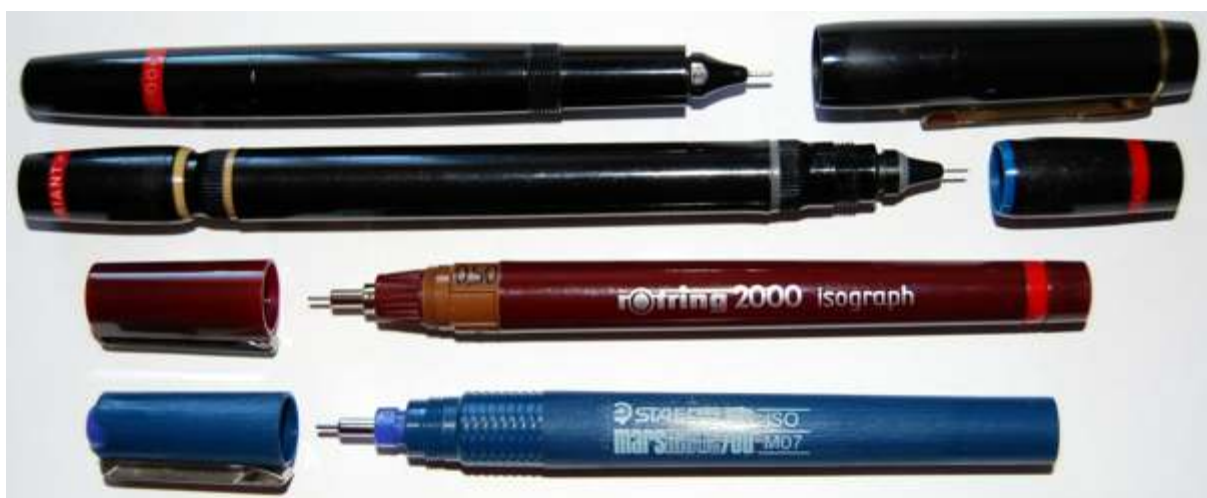
Fig. 232 Tubular nib pens: (a) Rotring Rapidograph fountain pen, (b) Rotring Variant double ended pen, (c) Rotring 2000 Isograph, (d) Staedtler MarsMatic 700 pen
