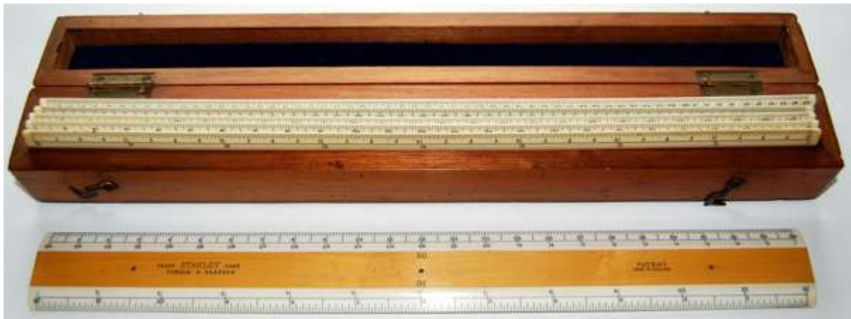
Fig. 64 Set of six W F Stanley celluloid edged boxwood surveyor's scales
