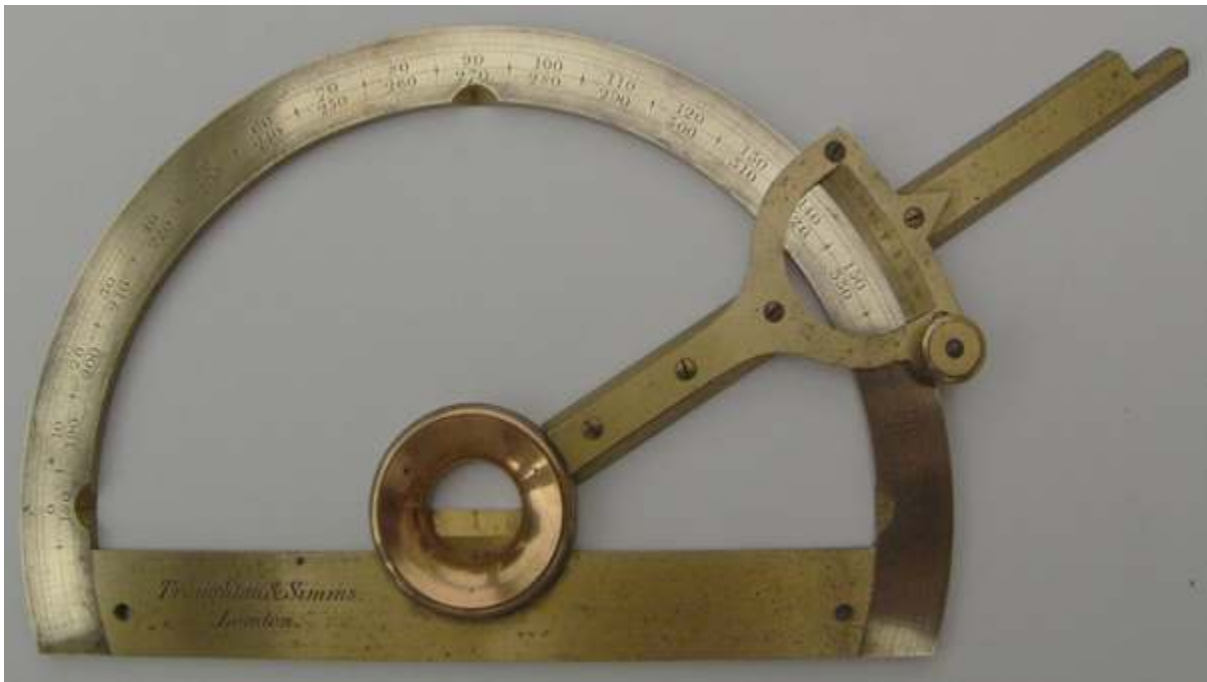
Fig. 43 Troughton & Simms, London single arm brass Vernier protractor
