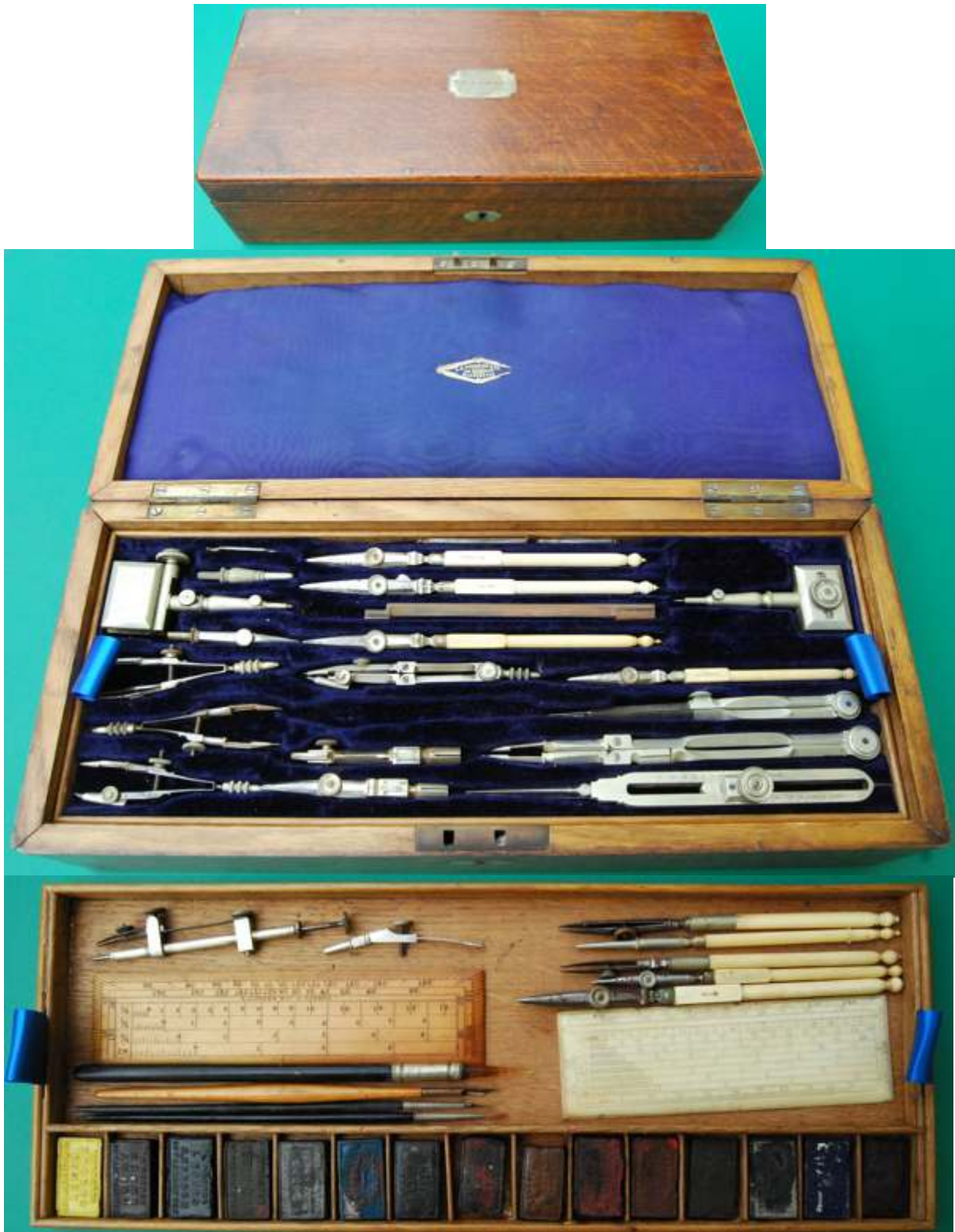
Fig. 305 A G Thornton, 109 Deansgate, Manchester three tier, 14 inch, oak case of electrum instruments Dating from ca.1890, the spring bows, bow compass and six-inch compass have screw-off points and the latter was made by W H Harling. At this date Alexander George Thornton did not make all of the instruments he sold and some were certainly bought in, so I am pretty certain these were all original to the set. Both Thornton and Harling listed these screw off points as their Improved Needle Points. In every case the spring bows have the same 3 knurled rings on the handle so they were most likely made by the same manufacturer. The lower tray contains a full set of colours by either Rowney or Winsor & Newton. As with many old sets spare space is filled with a miscellany of added items. The base contains a number of twelve inch scales.
