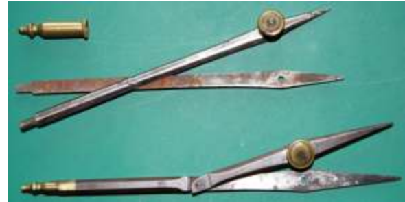
Fig. 80 Split steel pens opened for cleaning
