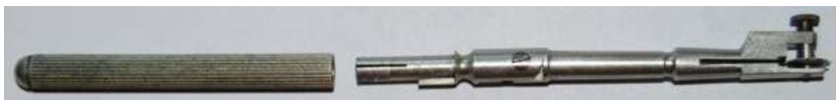
Fig. 203 Riefler dotted line pen disassembled to show spigot for fitting to compass leg. It has wheels for three types of dotted line.
