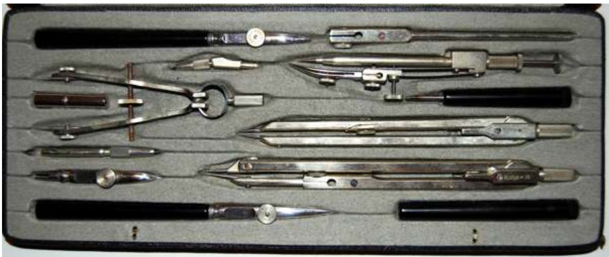
Fig. 281 E O Richter Precision No. 1836 drawing instrument set, ca. 1939
