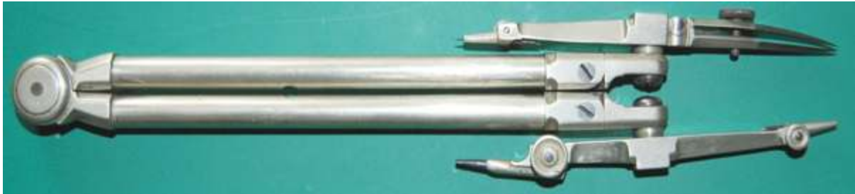
Fig. 100 Electrum telescopic turn-about compass
