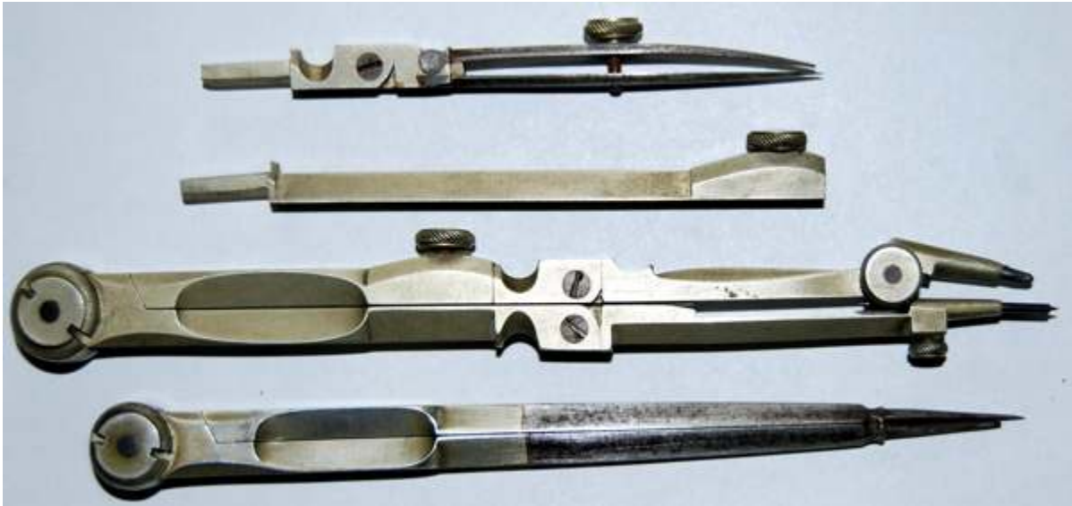
Fig. 184 Compass and divider made of German silver
