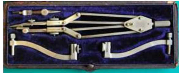
Fig. 238 Halden Vertical Compass in its case
