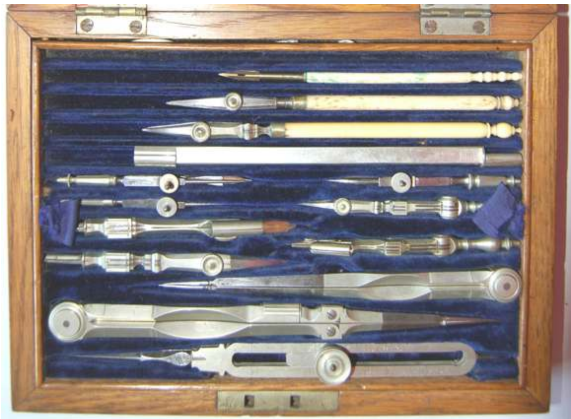
Fig. 264 Elliott Brothers set of electrum instruments in an electrum bound oak case
