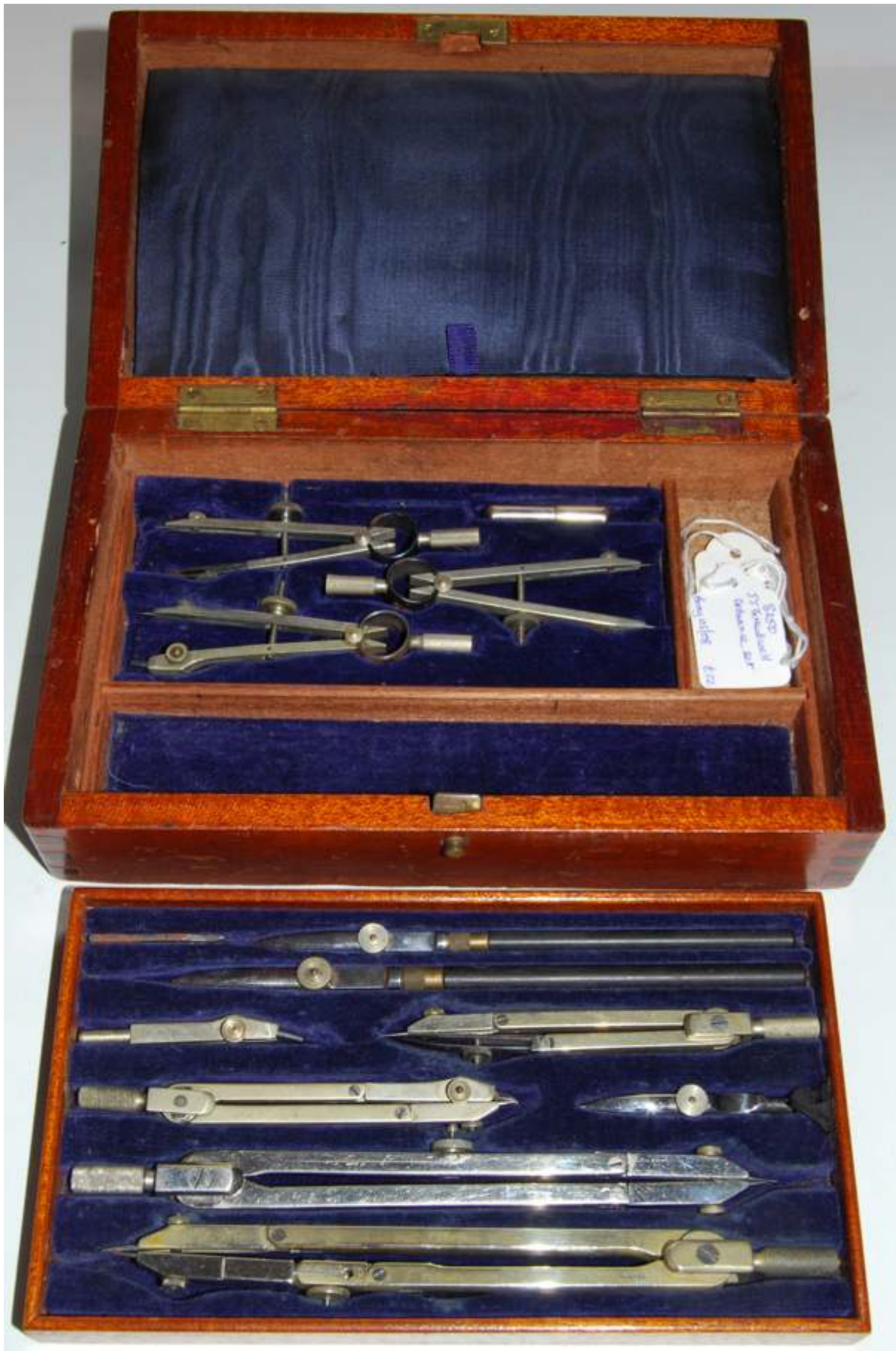
Fig. 278 J J Threadwell & Sons mahogany boxed set of instruments made for the British government. Some of the instruments are marked J J T Ltd beside the broad arrow. Note the mix of brass and nickel silver in this 1940s set due to material shortages.
