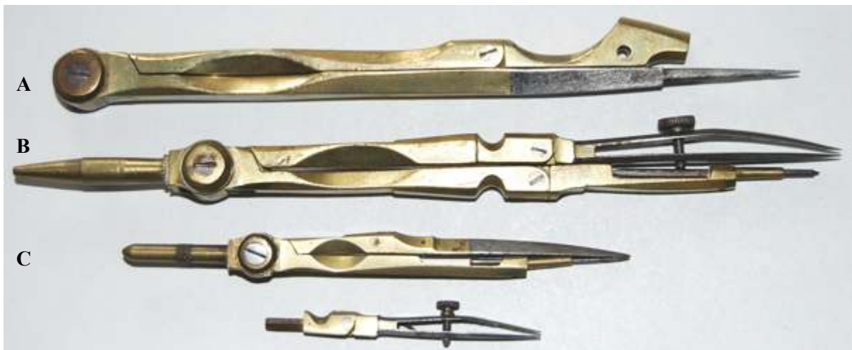
Fig. 169 Cheap French brass compasses, (a) school compass, (b) medium size compass, (c) smallest size
