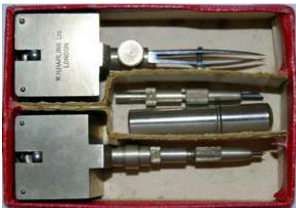
Fig. 118 Harling roller beam compass fittings
