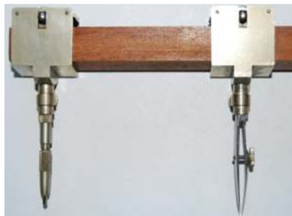
Fig. 119 Harling roller beam compass detail
