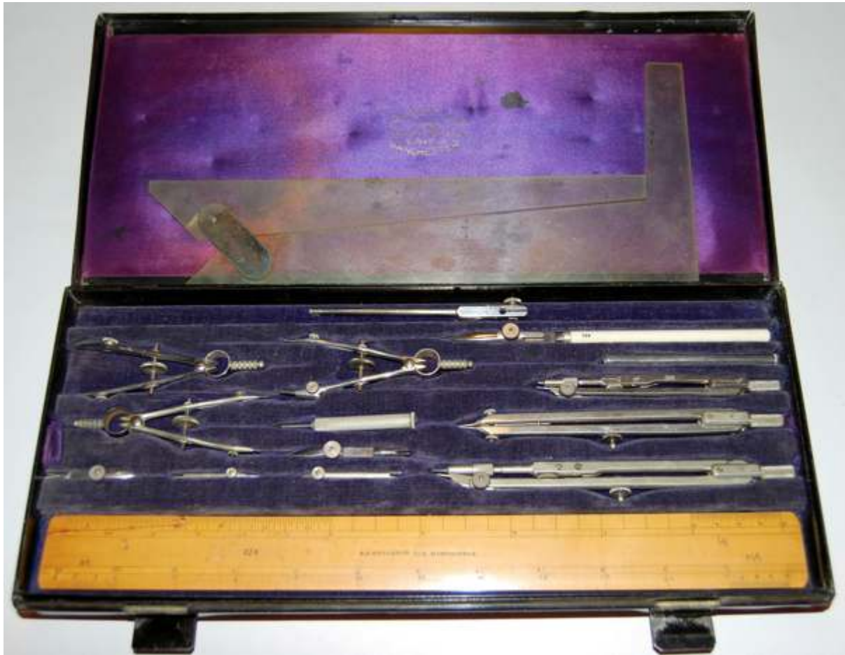
Fig. 320 A G Thornton 'Minerva Series' set in a metal case. The case and all the instruments and their parts in the tray are numbered '324'. Oddly there is no pocket for the lengthening bar, which rests in the long space at the back of the tray. The boxwood scale rule is an Armstrong type.
