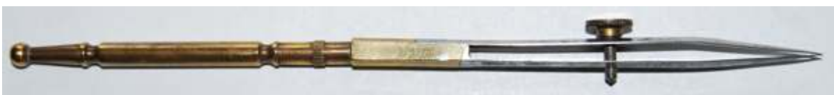
Fig. 190 Brass handled drawing pen from a Compassi di Milano set retailed by Gaetano Pistolesi, Cartoleria, Roma
