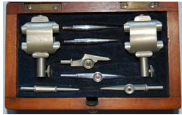
Fig. 105 Stanley patent 'La Trobe' beam compass fittings with 'flexible strap' for release
