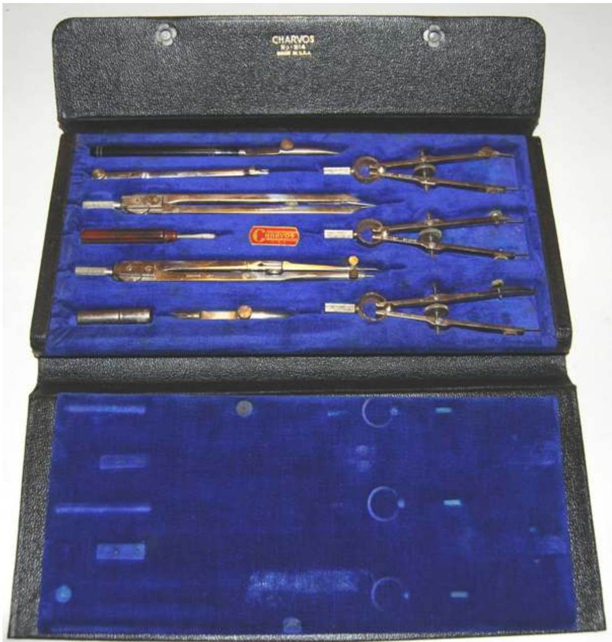
Fig. 312 Charvos No. 814 set, made in the USA. The set has a sturdy wallet case lined with blue velvet and probably dates from the 1940s. The instruments are plated, probably with chromium.
