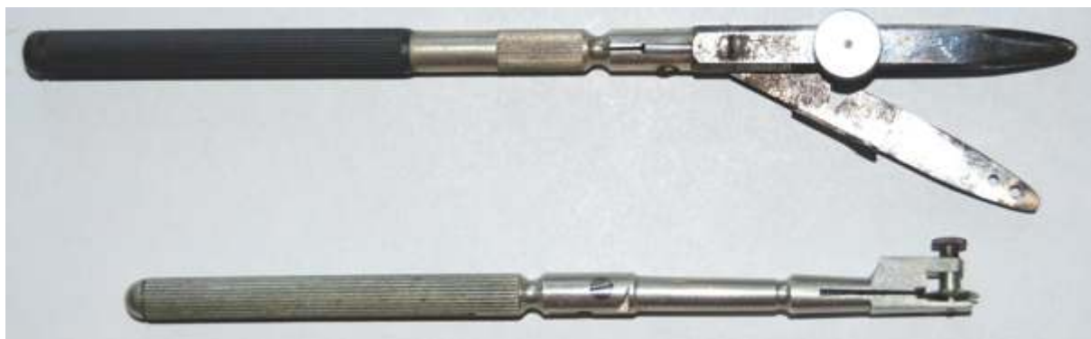
Fig. 202 Riefler pens: (a) three bladed pen showing centre blade opened for cleaning, (b) dotted line pen, 1930s. Both of these pens are actually compass fittings and can be detached from their handles, either of which could also be used with the compass ink point.. Both are also jointed.
