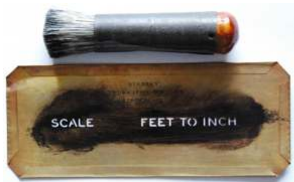
Fig. 134 Brass stencil plate and brush
