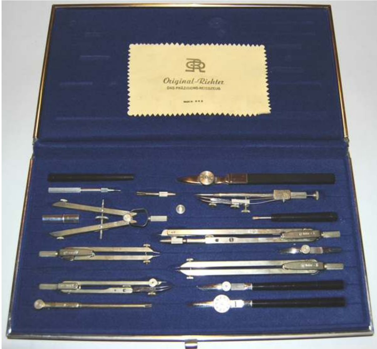
Fig. 317 Original Richter set made in East Germany, probably in the 1970s. The detail pen and the larger drawing pen have large, graduated thumb wheels for setting the line thickness. The case is steel, covered with leather and lined with blue velvet, which is padded inside the lid with foam.
