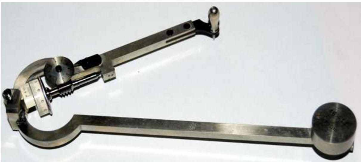
Fig. 139 Amsler type 2 fixed scale polar planimeter no. 22935 dating from ca. 1896
