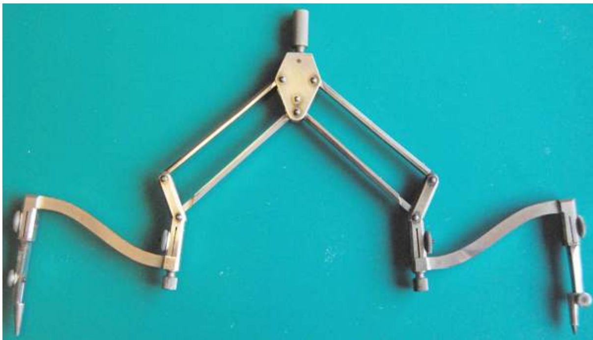
Fig. 240 Halden Vertical Drawing Compass with lengthening bars fitted. The compass was made of finest quality electrum.
