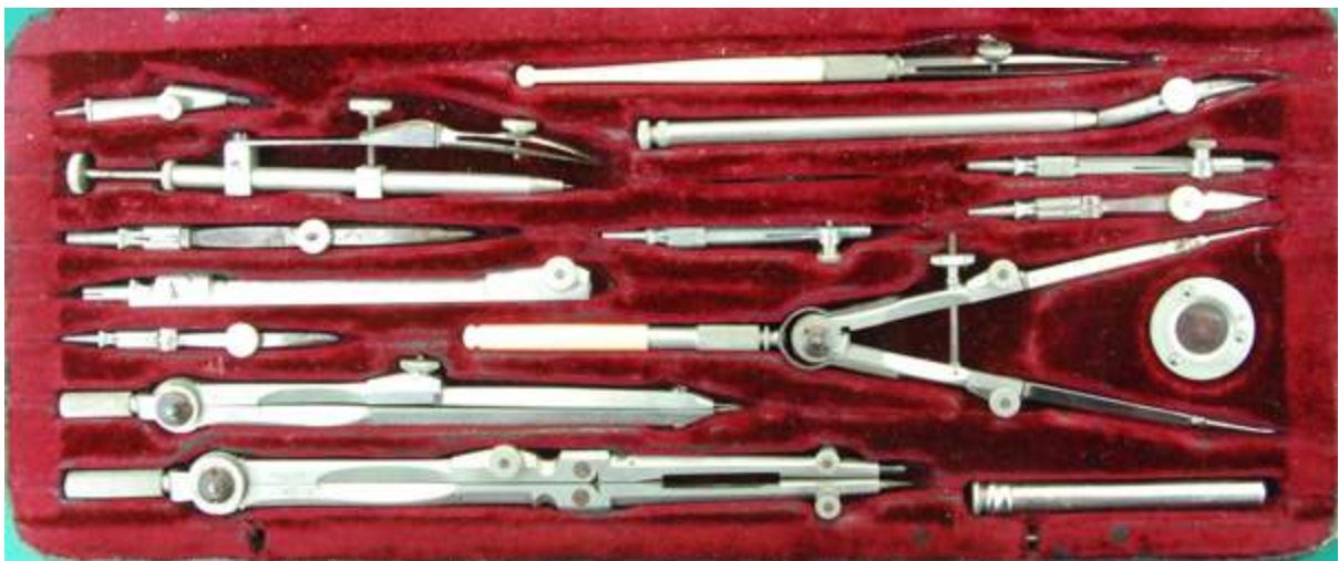
Fig. 288 Kern set dating from ca.1910. Note the unusual spring bow that has two pencil points and two pen points as well as the two plain points so it can be used to draw pairs of ink and pencil lines as well as being used as a compass
