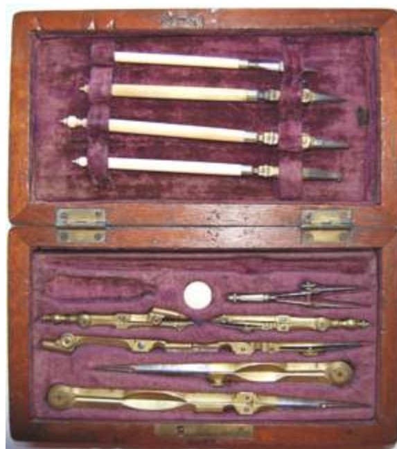
Fig. 261 William Elliott, 268 High Holborn, set of brass drawing instruments in a mahogany case, dating from 1835-49. Missing lengthening bars and compass key
