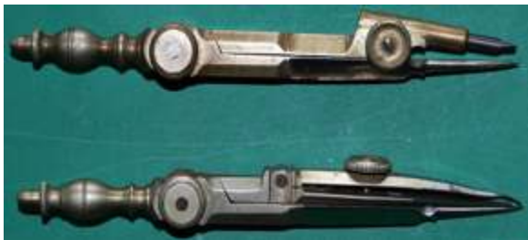
Fig. 14 Electrum bows by Elliott Brothers which have no leg joints
