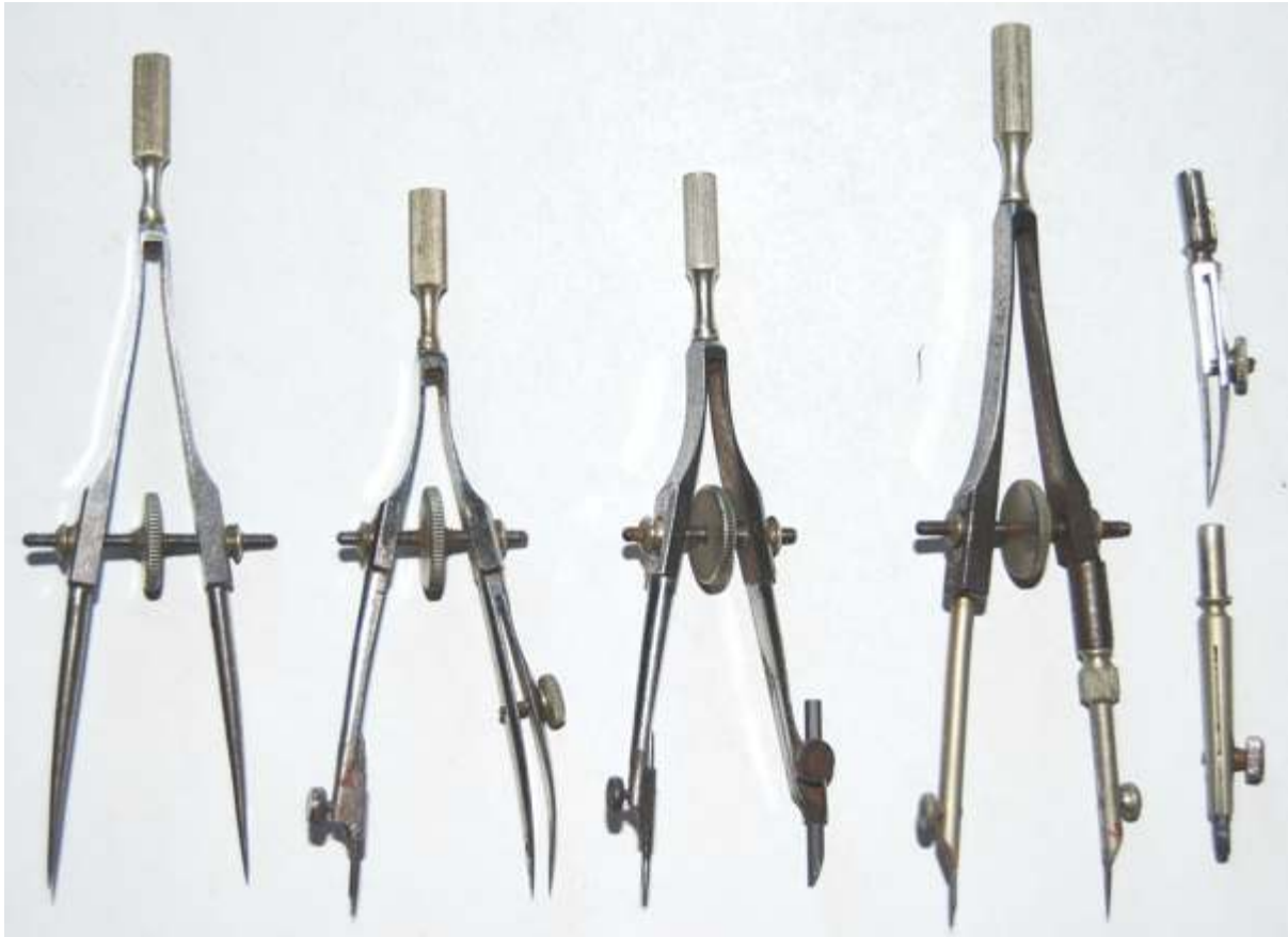
Fig. 205 Spring bows from Riefler sets. The first three are ca. 1900/1910, the last is from the 1930s and has interchangeable divider, ink and pencil points.
