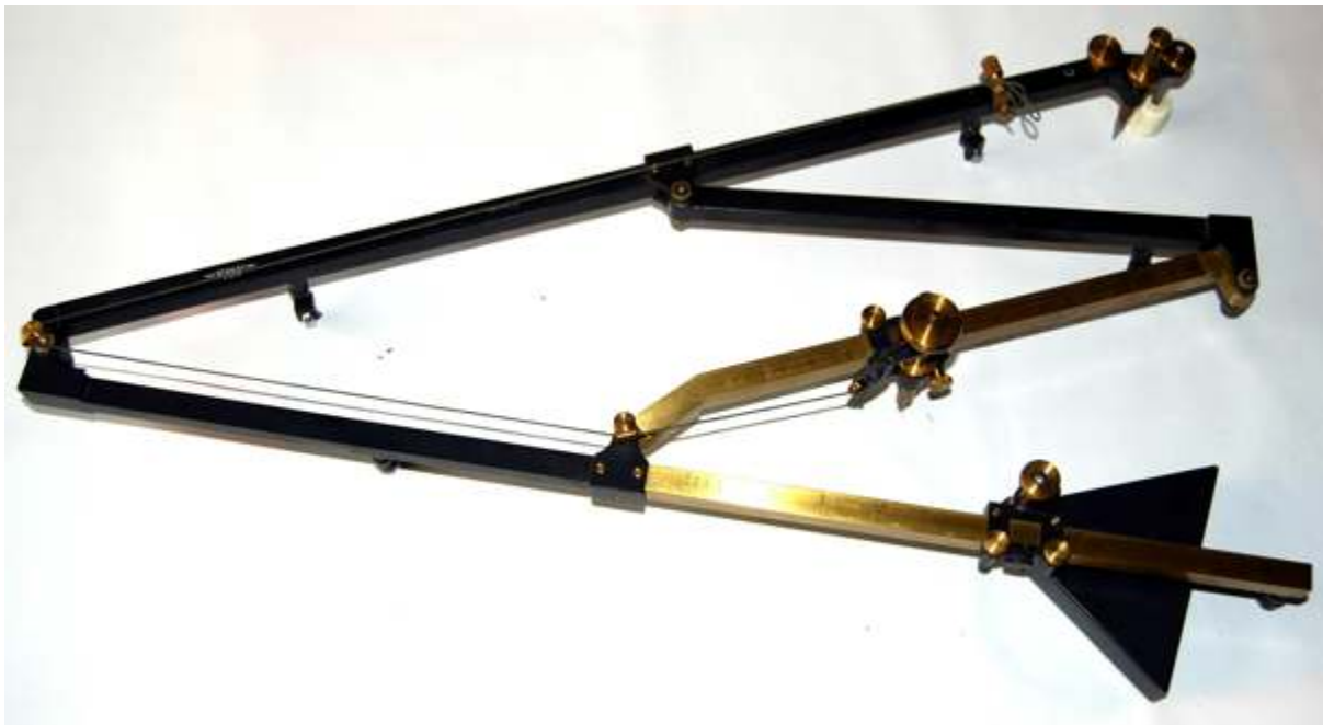
Fig. 148 W F Stanley 26 inch pantograph with box section arms, probably early 20th century
