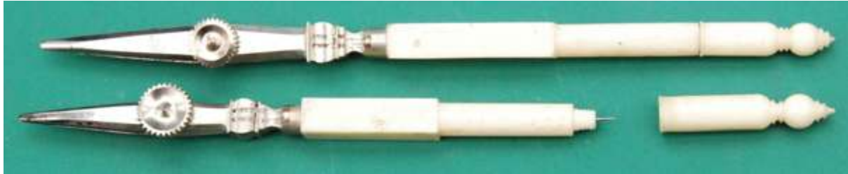
Fig. 191 Japanese ruling pens with removable caps revealing pricker in handle
