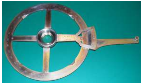
Fig. 44 Stanley electrum Vernier protractor
