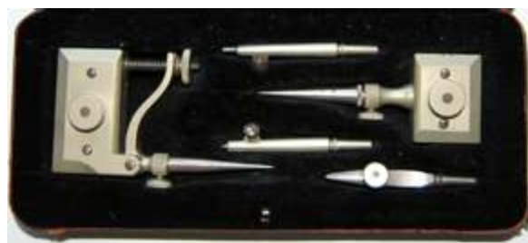
Fig. 111 Beam compass fittings by Riefler, Germany
