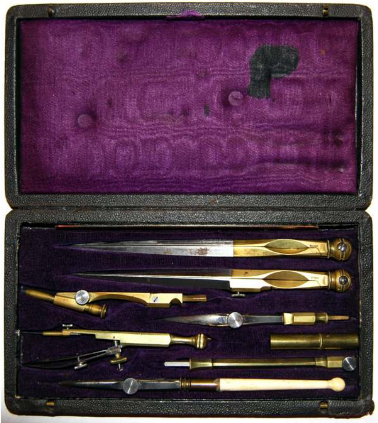
Fig. 308 A small set of French brass instruments with some unusual features. The compass and dividers have spherical heads and are stamped 'Déposé' indicating that the design was registered. The pencil point has a separate lead holder.
