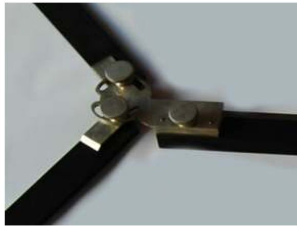
Fig. 158 Centrolinead joint detail
