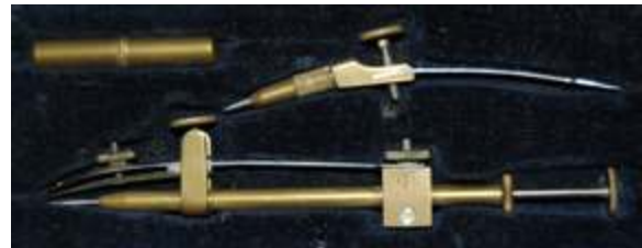
Fig. 280 Richter Industrie brass drop bow compass
