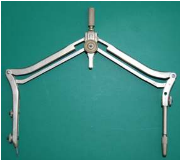
Fig. 242 Original Lotter Parallel Compass
