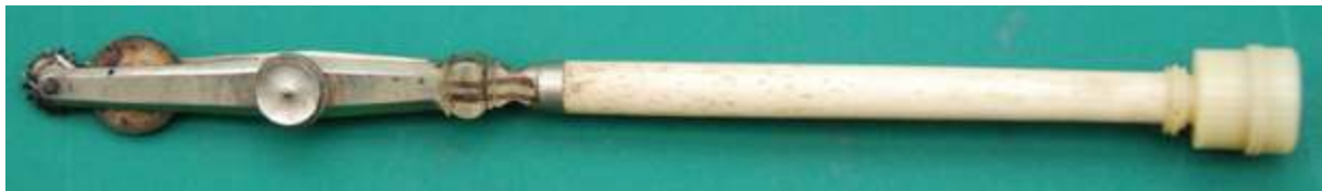
Fig. 192 Japanese dotted line pen with revolving ink feed wheel
