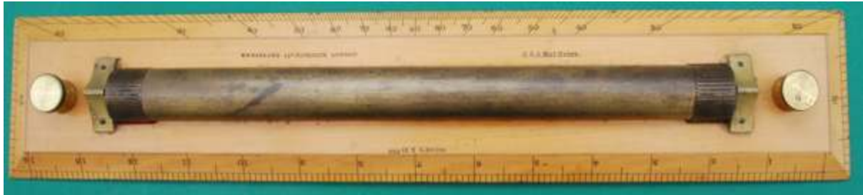
Fig. 72 W H Harling boxwood & brass 15 inch rolling 'Capt. Field's Improved' parallel rule
