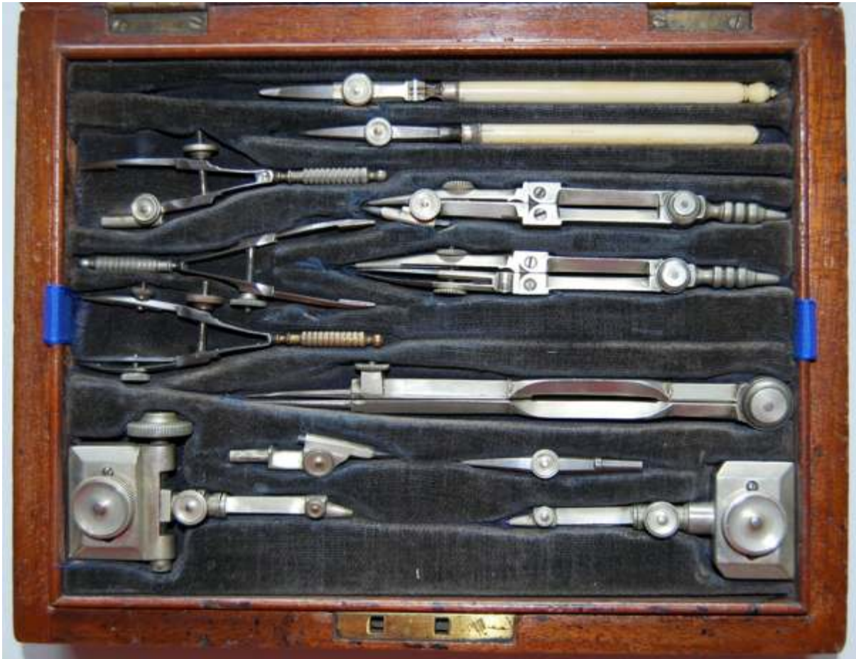
Fig. 274 Halden hand made English drawing instruments dating from 1925. The set is unusual as it has beam compass fittings instead of a six inch compass half set. The case is mahogany.
