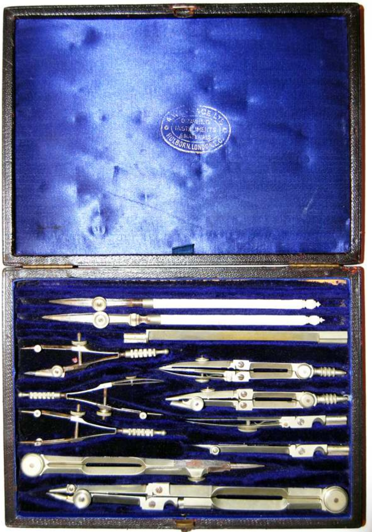
Fig. 302 Full set of electrum drawing instruments in a Morocco, snap fastening case retailed by A W Gamage, Holborn, London EC, ca. 1900 The compass and spring bows have ordinary needle points, whilst the pen and pencil bows have nut and bolt needle points.
