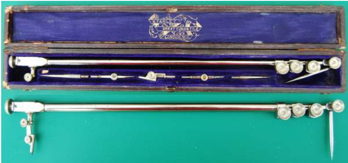
Figs. 101 & 102 W F Stanley, Great Turnstile, London, tubular telescopic beam compass, ca. 1900
