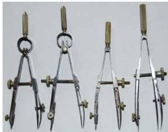
Fig. 175 German and Swiss ink spring bows - from the left: (a) Schoenner, (b) Schoenner, (c) Eugene Dietzgen, (d) Kern (Note: three different types of needle fastening)
