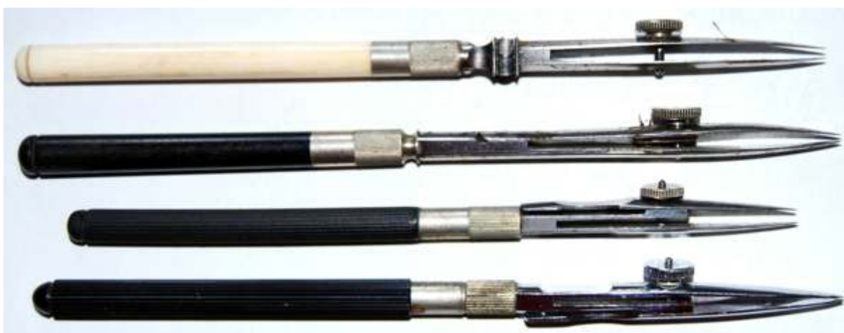
Fig. 199 Riefler round system pens: (a) lifting nib and ivory handle, ca. 1900/1910 (b) earliest type of cross joint pen, ca. 1900/1910, (c) second type of cross joint pen, ca. 1930, (d) third type of cross joint pen, 1950s
