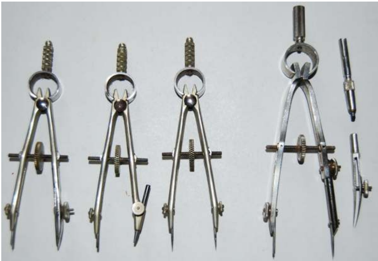
Fig. 212 'C' spring bows: (a), (b), (c) Thornton Minerva series, (1930s); (d) Nestler
