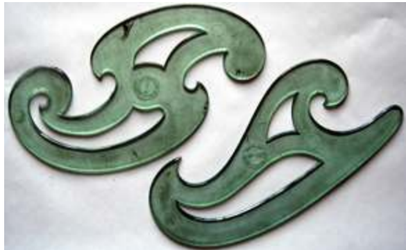
Fig. 77 'Simplon' transparent plastic French curves
