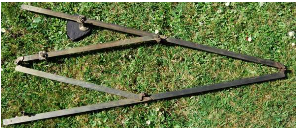
Fig. 147 Elliott & Sons 36 inch brass pantograph dating from 1850 - 1853
