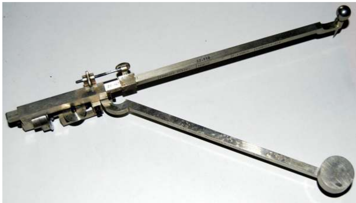
Fig. 140 Amsler type 4 adjustable scale polar planimeter no. 15090 dating from ca. 1888
