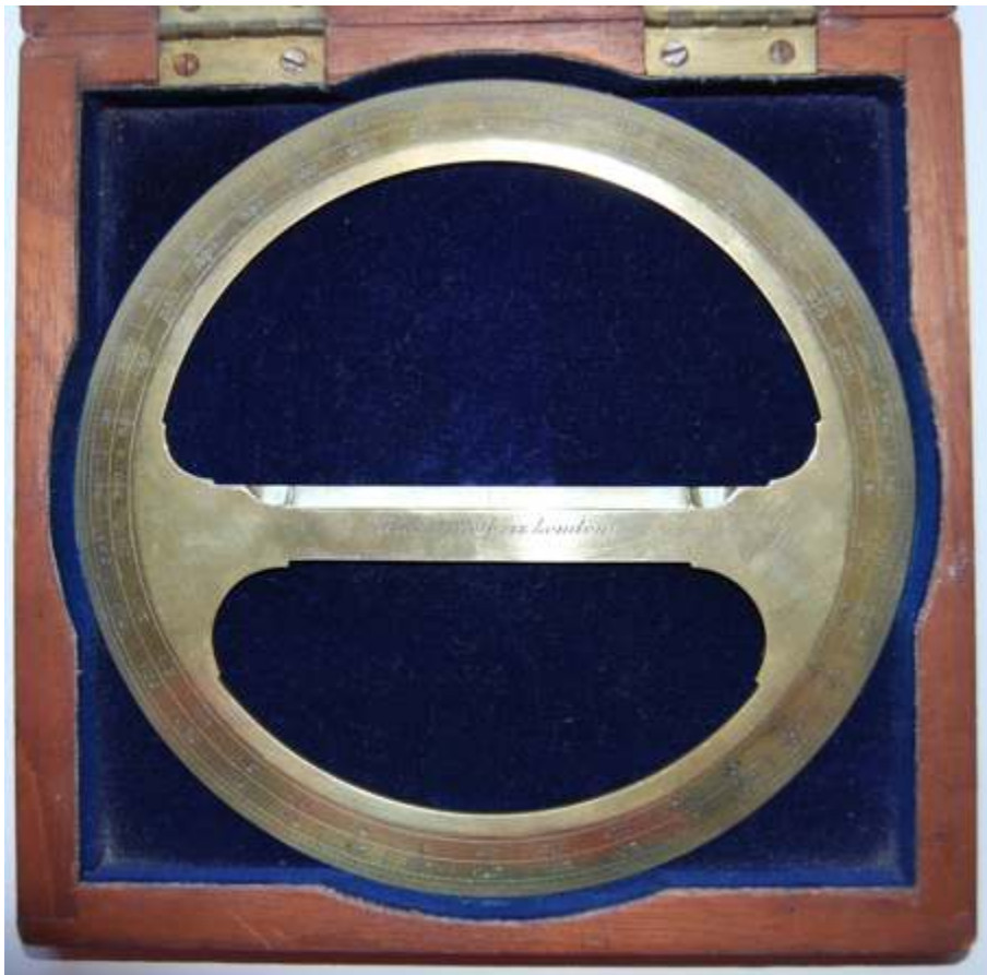
Fig. 263 Elliott Brothers, London six inch brass protractor and mahogany case
