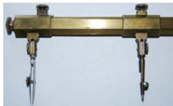
Fig. 107 Detail of Wichmann beam compass
