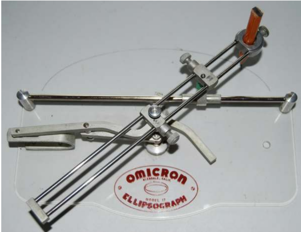
Fig. 150 Omicron Model 17 Ellipsograph, 1950s, aluminium, steel and acrylic.
