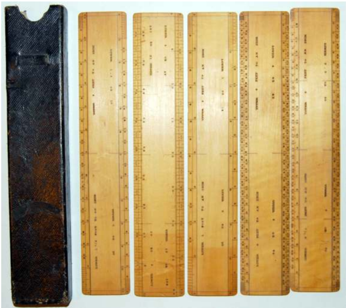
Fig. 322 Set of five 8 inch boxwood architect's scales signed Reeves & Sons, Cheapside, London in a leather and card case.
