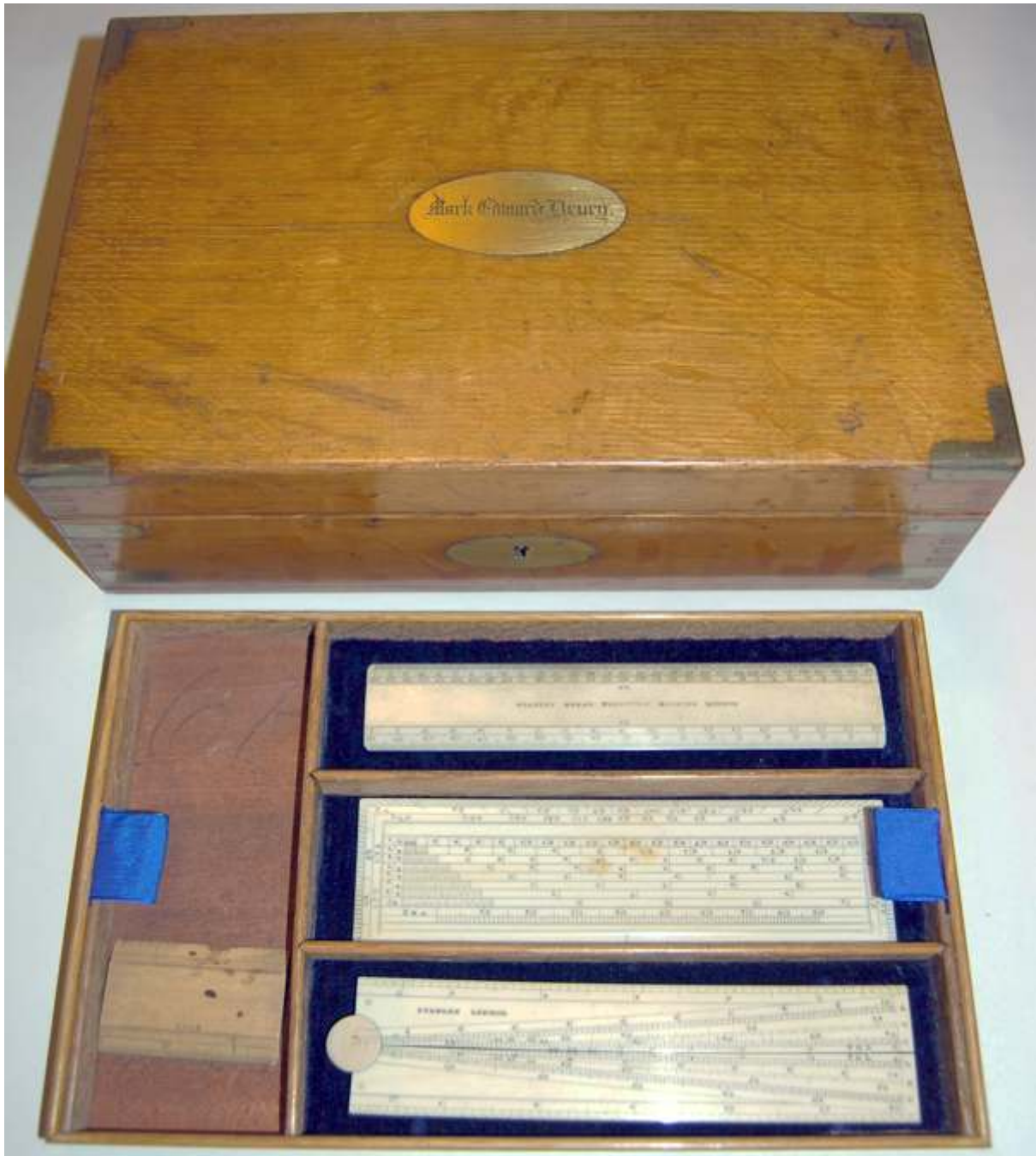
Fig, 299 W F Stanley ten inch electrum bound oak case of electrum drawing instruments, ca, 1880 This view shows the case exterior and the lower tray with the sector, protractor and scale rule. The cartouche is elaborately engraved with the name of the original owner, 'Mark Edward Drury'.
