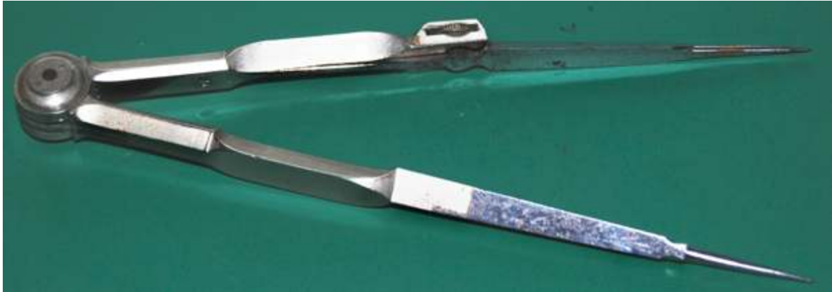
Fig. 9 Hair spring divider with captive adjusting screw, earlier type with adjusting screw in the middle of the leg rather than near the point.
