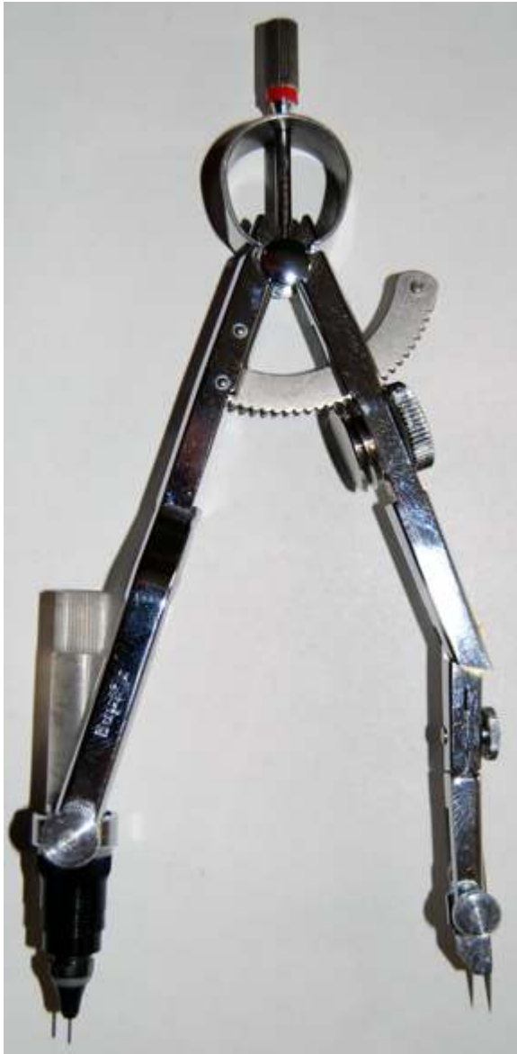
Fig. 233 Rotring 532 101 Master Bow Compass fitted with a Variant pen unit
