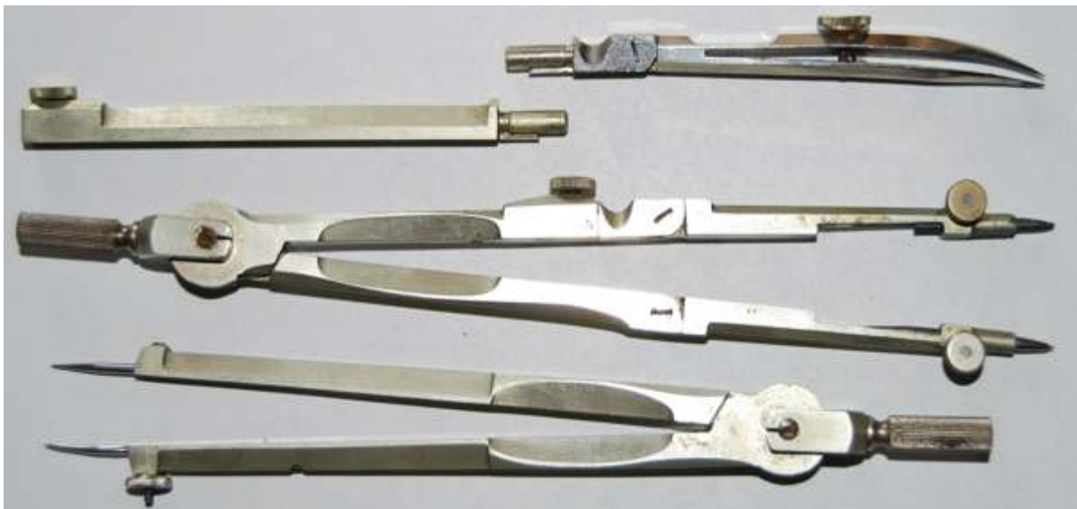
Fig. 181 German made compass and hair divider from a Keuffel & Esser Doric set. The compass and divider heads have a hidden straightening device. The compass ink and pencil points have a circular cross section spigot with a steel feather. The socket has a clamping screw directly pressing on the spigot. unlike the Schoenner, Post and Kern examples where the socket is slit and the clamping screw compresses the socket around the spigot.
