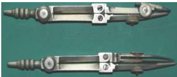
Fig. 15 Halden double jointed bow compasses
