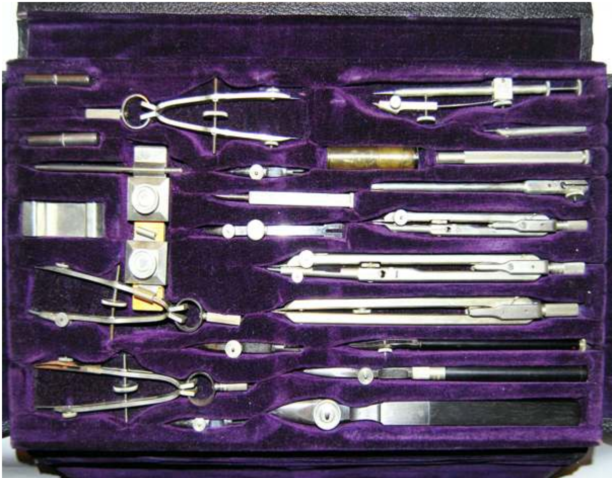
Fig. 311 Friedmann Brothers Drawing Instrument Co., New York No. 23A set dating from ca. 1935 in a leather wallet case containing their Universal Micromatic Beam Compass. It retailed at $33 with a discount price of $16.50 according to their price list. This was the largest set in the catalogue. The nickel silver instruments were made in Germany.
