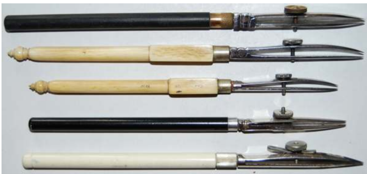
Fig. 211 Flat system pens: (a) Cooke, Troughton & Simms, lifting nib, (b) Thornton, ivory handle & lifting nib (1939), (c) Thornton, ivory handle & spring nib (1939), (d) Nestler, cross-joint nib, (e) Ecobra, white plastic handle, spring nib with release
