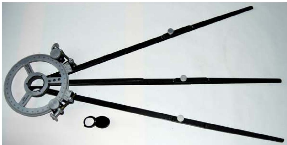
Fig. 154 Heath & Co, London SE9, station pointer, aluminium & steel, mid-20th century, No. 5157
