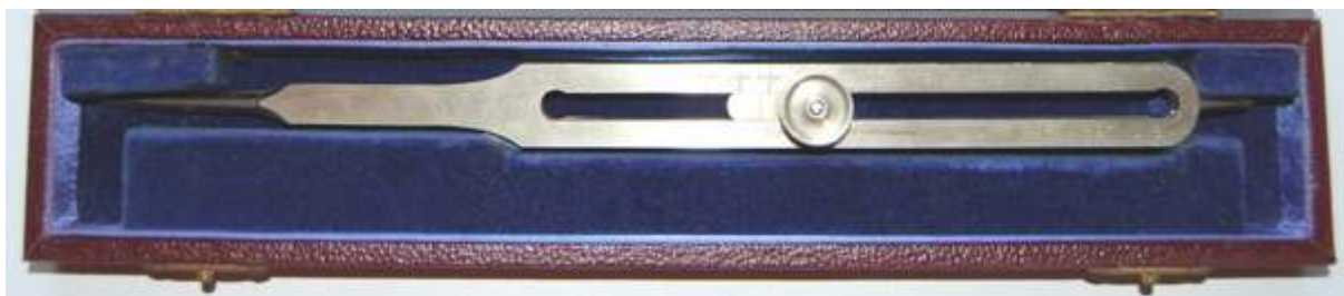
Fig. 277 J J Threadwell & Sons Ltd. ten inch proportional divider, late 20th century
