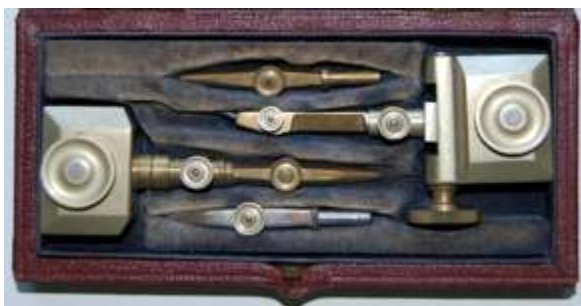
Fig. 110 English made Swiss pattern beam compass
