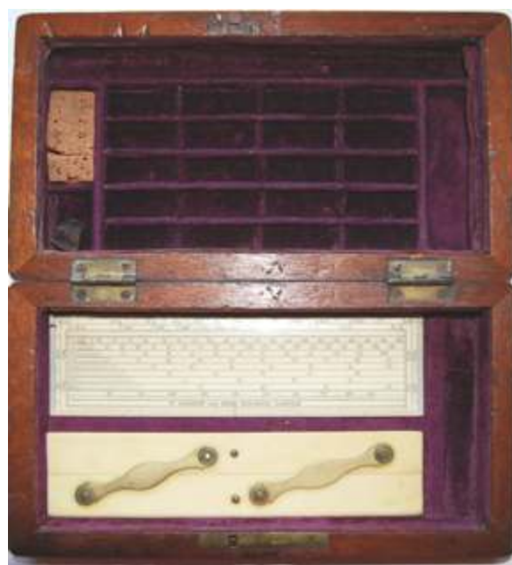
Fig. 262 William Elliott box with trays removed to show ivory items and spaces for water colours and brushes
