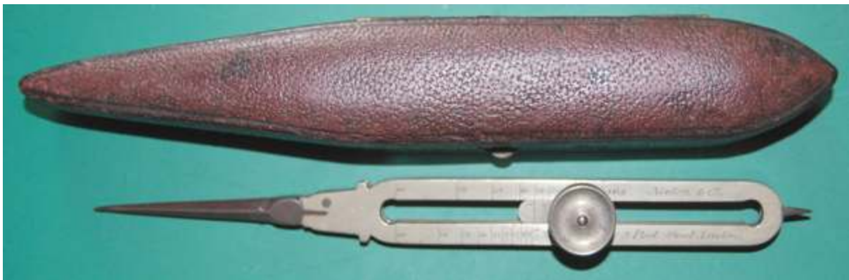
Fig. 121 Six inch electrum proportional dividers and fitted case by Newton & Co., 3 Fleet Street, London
