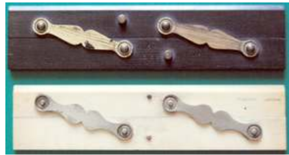
Fig. 70 Six inch parallel rules, the upper in ebony and brass, the lower by Stanley in ivory and electrum
