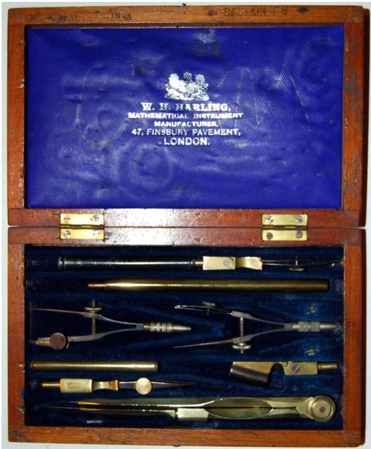
Fig. 326 W H Harling patent cone fitting set comprising patent cone fitting compass with ink, pencil and plain points, and lengthening bar; pen handle; ink and pencil spring bows. These brass instruments in a simple mahogany box were designed for school use. They are robust and serviceable, yet they were cheap to produce.
