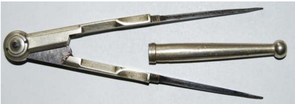
Fig. 188 Italian dividers with the sheath removed and opened to show the long joint and the screw thread for attaching the sheath.
