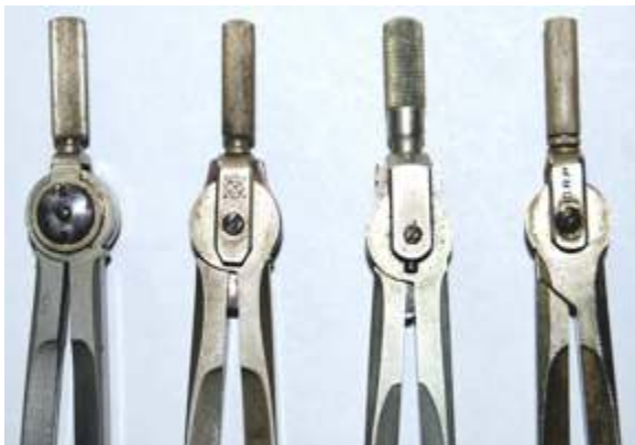
Fig. 182 Head joints - from the left: (a) Kern, (b) Schoenner, patented 17.3.1903, (c) Post's pivot joint with clamping screws from the College set, (d) Eugene Dietzgen
