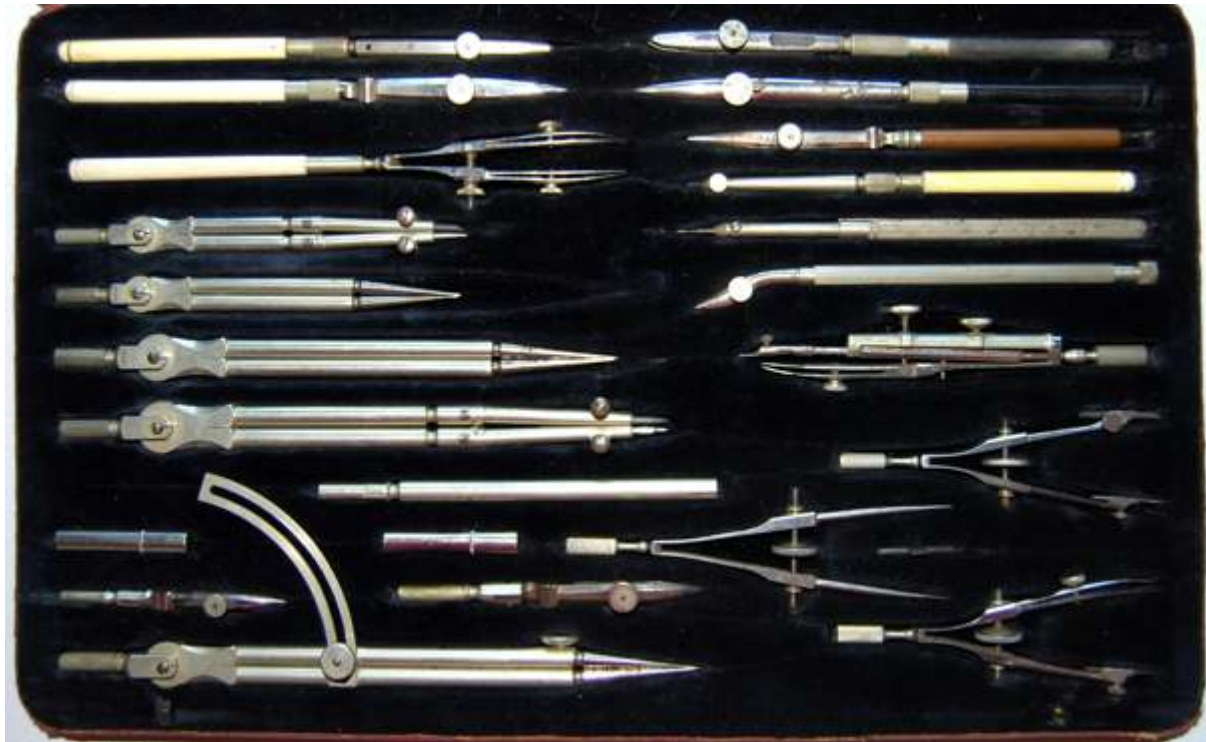
Fig. 284 Early 20th century set of Riefler round system drawing instruments. The set also includes an ex-centrolinead and a horn centre behind a flap in the lid. There was also a protractor, now missing.
