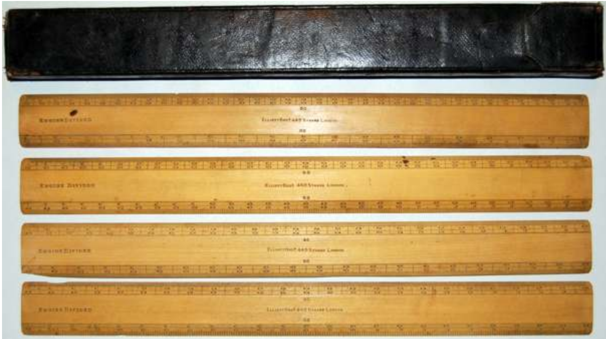
Fig. 321 Set of four 12 inch boxwood chain scales signed Elliott Bros., 449 Strand, London in a leather and card case. Like many scales these have the original owner's name stamped on the reverse. The maker would do this for a small extra charge.
