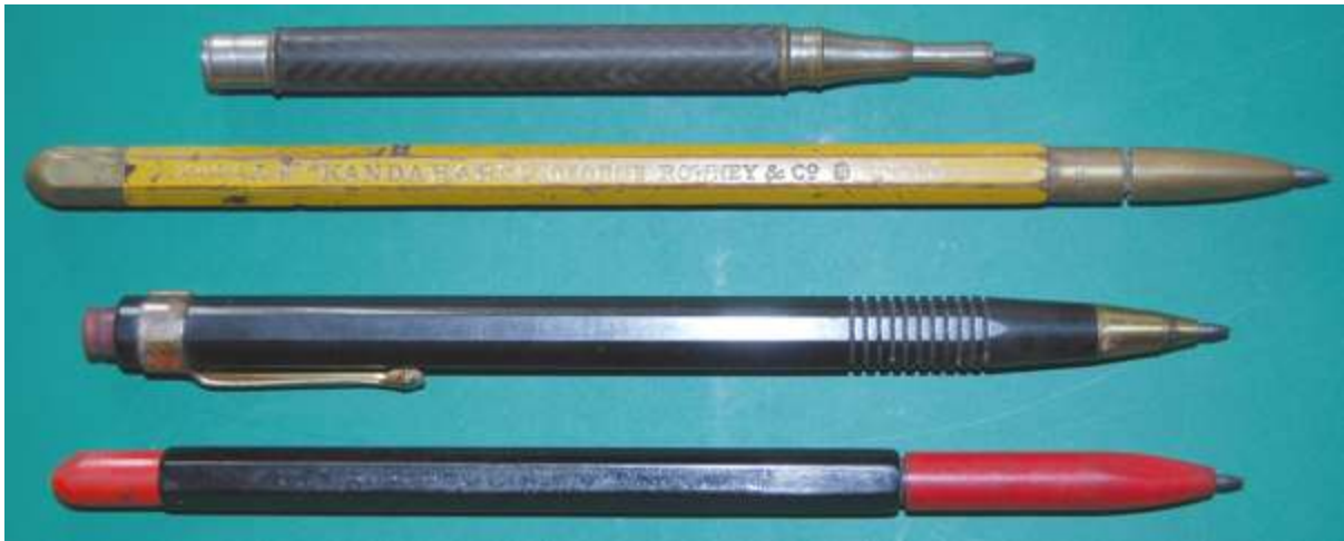
Fig. 127 English lead holders: (a) Propelling pencil for artist's leads; (b) Rowney & Co twist lock clutch pencil; (c) Rexel push button clutch pencil; (d) Chisilient draughtsman's pencil
