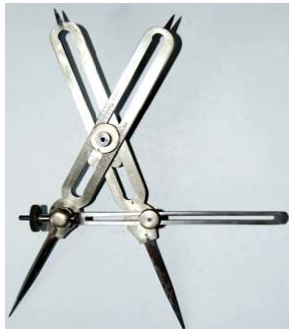
Fig. 273 Halden six inch proportional dividers with adjusting bar. These differ from those pictured earlier and the adjusting bar is steel.
