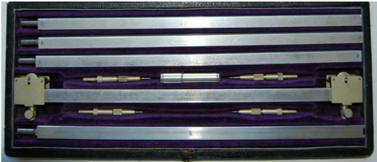
Fig. 117 'New Portable Beam Compass', unsigned but probably made by W H Harling, 1930s
