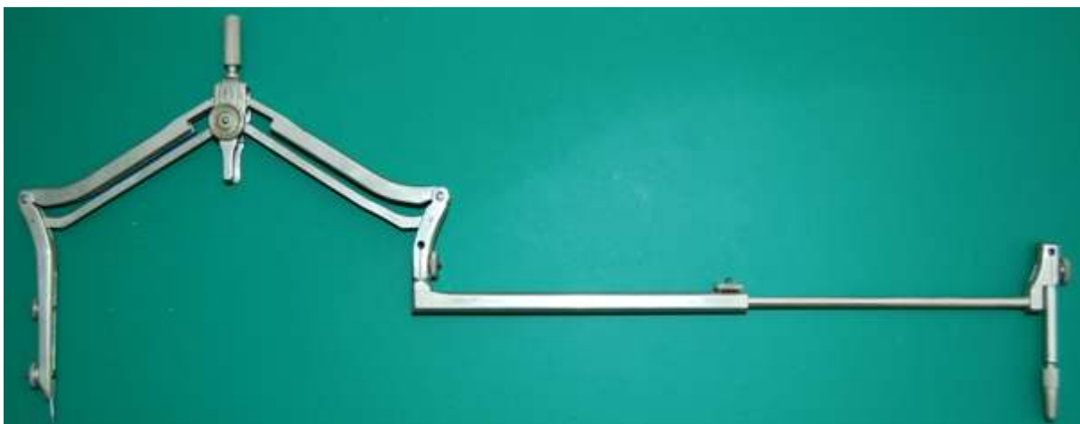
Fig. 243 Original Lotter Precision Parallel Compass with its telescopic lengthening bar fitted and fully extended
