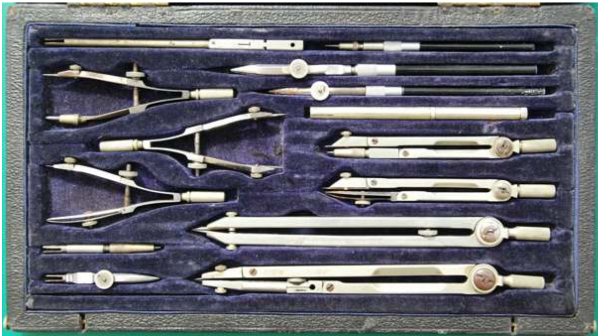
Fig. 275 Halden flat pattern set, probably ca. 1920. This is a variant of the British Empire pattern.
