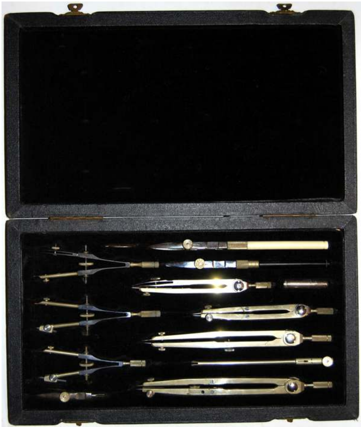
Fig. 313 Lee Guinness S902 flat system set, ca. 1950. Besides making round system instruments based on the Riefler design, Lee Guinness also made two qualities of flat system instruments, of which this is an example of the better quality. Both pens have cross joint nibs. The black handled one is a Lee Guinness replacement and has a pricker on the ed of the handle, which unscrews..
