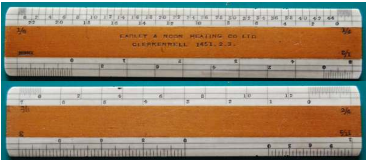
Fig. 66 Boxwood and celluloid six inch Armstrong scale
