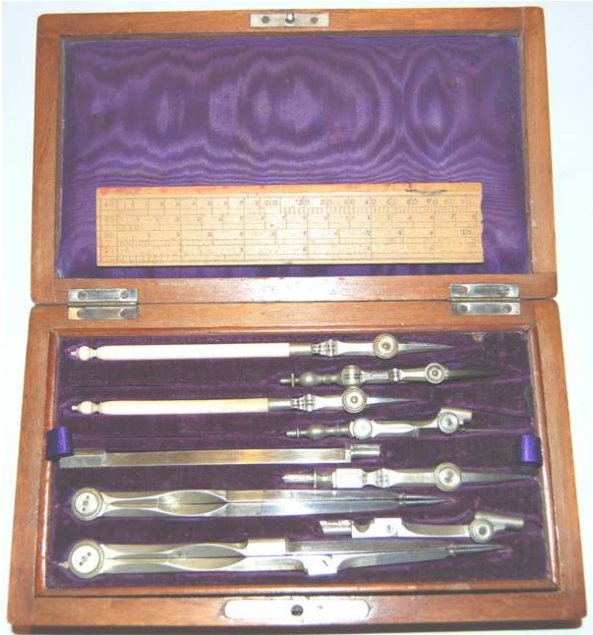
Fig. 301 A late 19th century set of electrum instruments in a mahogany case with a domed lid. The set is unsigned. The compass has plain points yet is double jointed. There are also two boxwood plain scales (only one shown)
