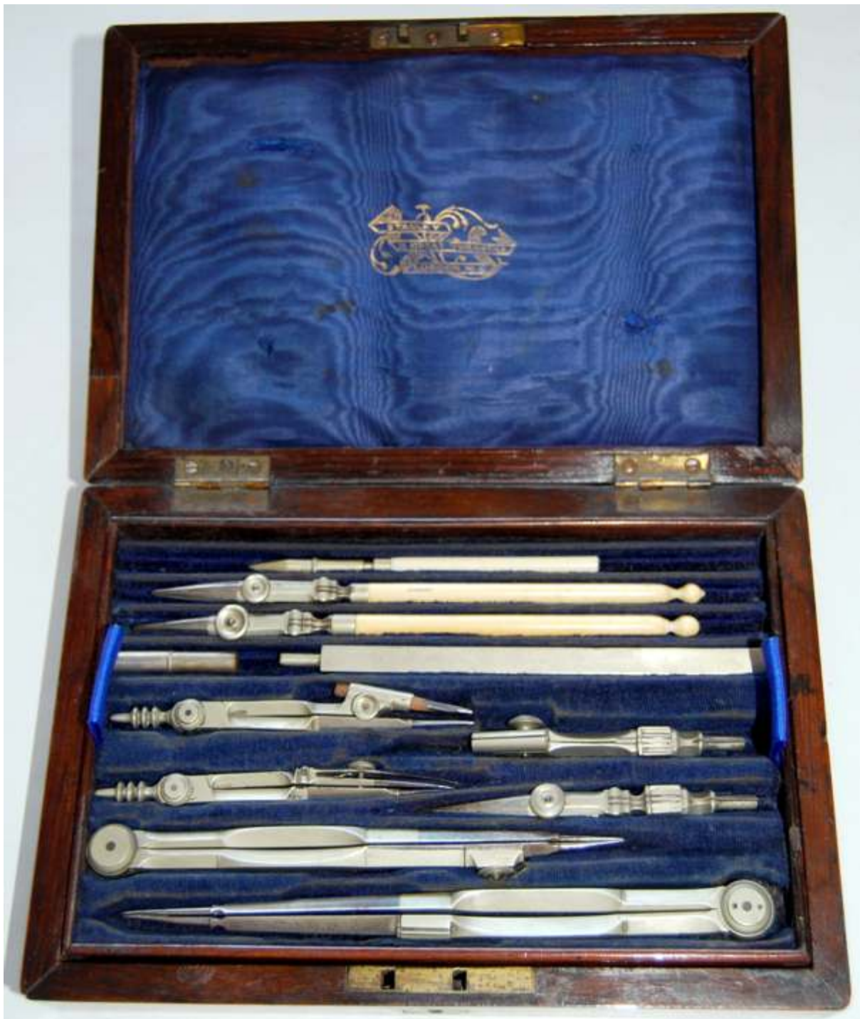
Fig. 254 Rosewood veneered case of electrum drawing instruments by W F Stanley, late 19th century. This set of electrum instruments is one of Stanley's cheaper products. Neither the compass, nor the bows are double jointed and the slip joint for the compass points is not Stanley's improved pattern. Also the compasses have plain points and are fitted for lead pencils rather than pencil leads.
