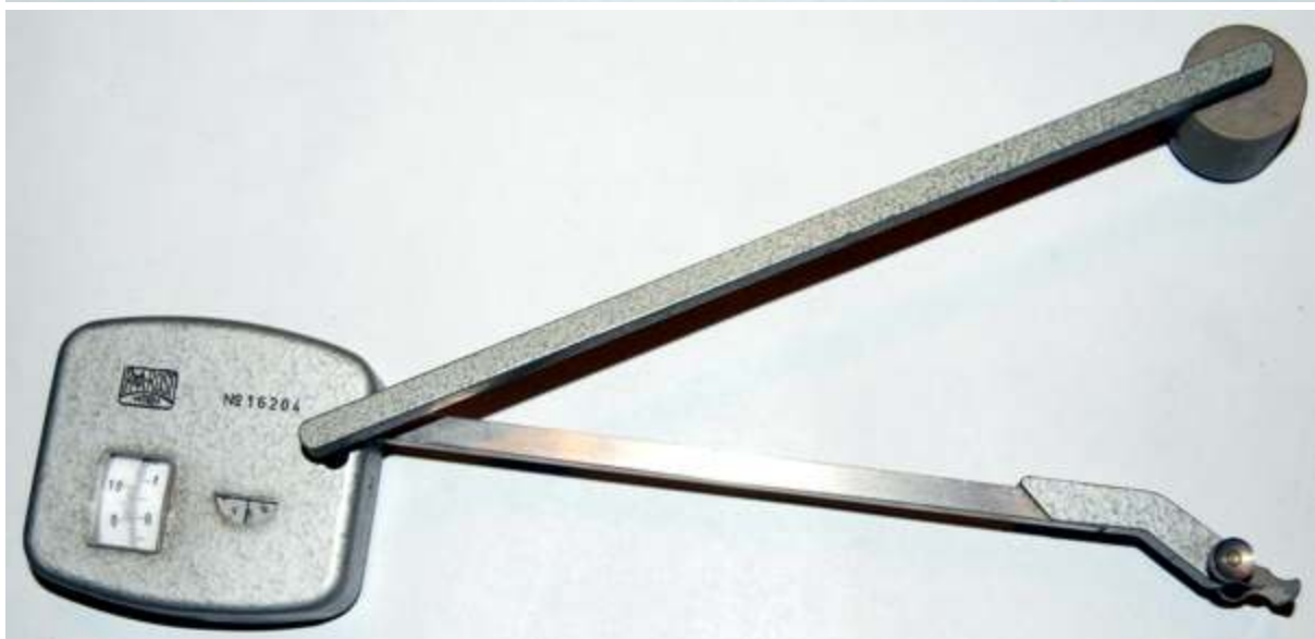
Fig. 323 Compensating planimeter by R & A Rost, Vienna dated 1967. Serial No. 16204. Black leatherette covered, red velvet lined case, calibration chart and checking bar. The planimeter has a grey crackle finish.
