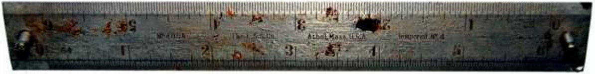
Fig. 250 No. 405A The L.S.S.Co., Athol, Mass., USA Tempered No. 4 patent tilting rule
