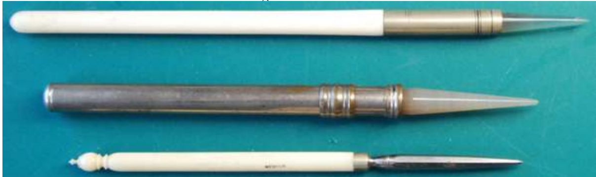
Fig. 133 Tracers: (a) ivory handle with agate point; (b) metal handle with retractable agate point; (c) ivory handle with steel point
