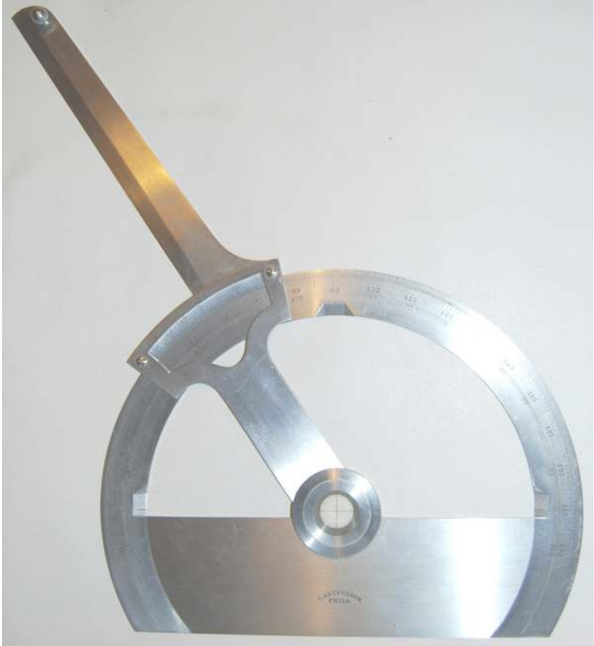
Fig. 318 Theo Alteneder eight inch stainless steel Vernier protractor. The Vernier reads to one minute.
