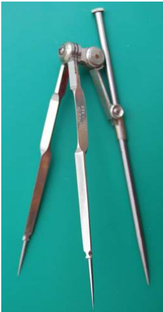
Fig. 138 Heath & Co triangular divider
