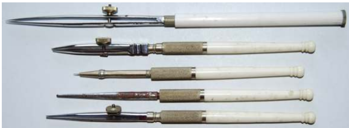
Fig. 276 J J Threadwell & Sons Ltd. (a) lithographic pen, (b) lifting nib pen, (c) pricker, (d) tracer, (e) fine line pen, late 20th century
