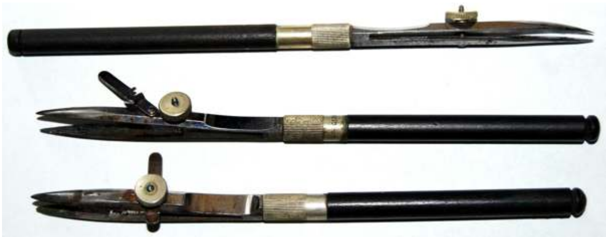
Fig. 180 German spring blade pens: (a) Eugene Dietzgen, (b) Schoenner from 1912 set, (c) Schoenner The two Schoenner pens have a release to open the blades for cleaning. The upper pen has a release patented February 4th 1904 with a separate pivot. The lower one pivots about the adjusting screw. all three have vulcanite handles although aluminium was also used.
