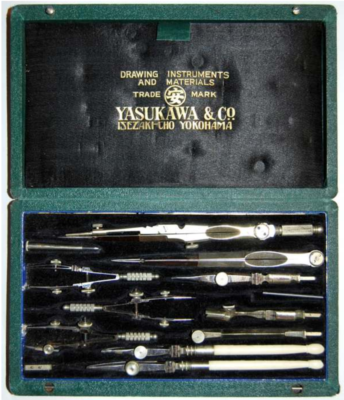
Fig. 307 Yasukawa & Co., Isezaki-cho, Yokohama, Japan set of nickel silver instruments in a green, cloth covered, pin lock case. This set is a mixture of English and French styles. The spring bows are English pattern but the compass and pens imitate French instruments. The compass pencil point has a separate lead holder.
