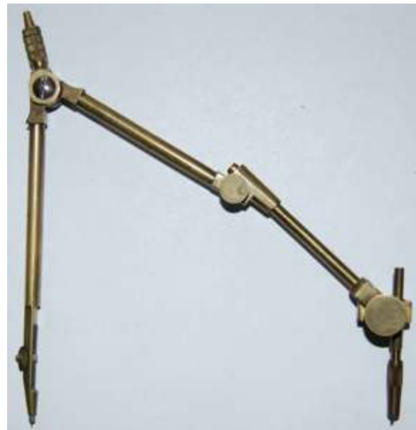
Fig. 248 Jackson Bros. compass with lengthening bar fitted
