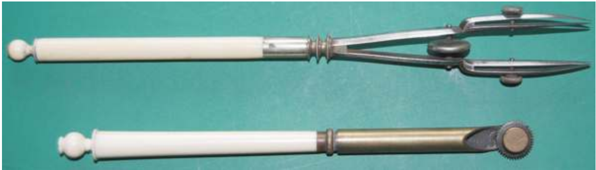
Fig. 172 French ivory handled road pen and dotted line pen. The finial on the dotted line pen is a particularly fine example of that seen also on the road pen and pen 'b' in Figure 165.
