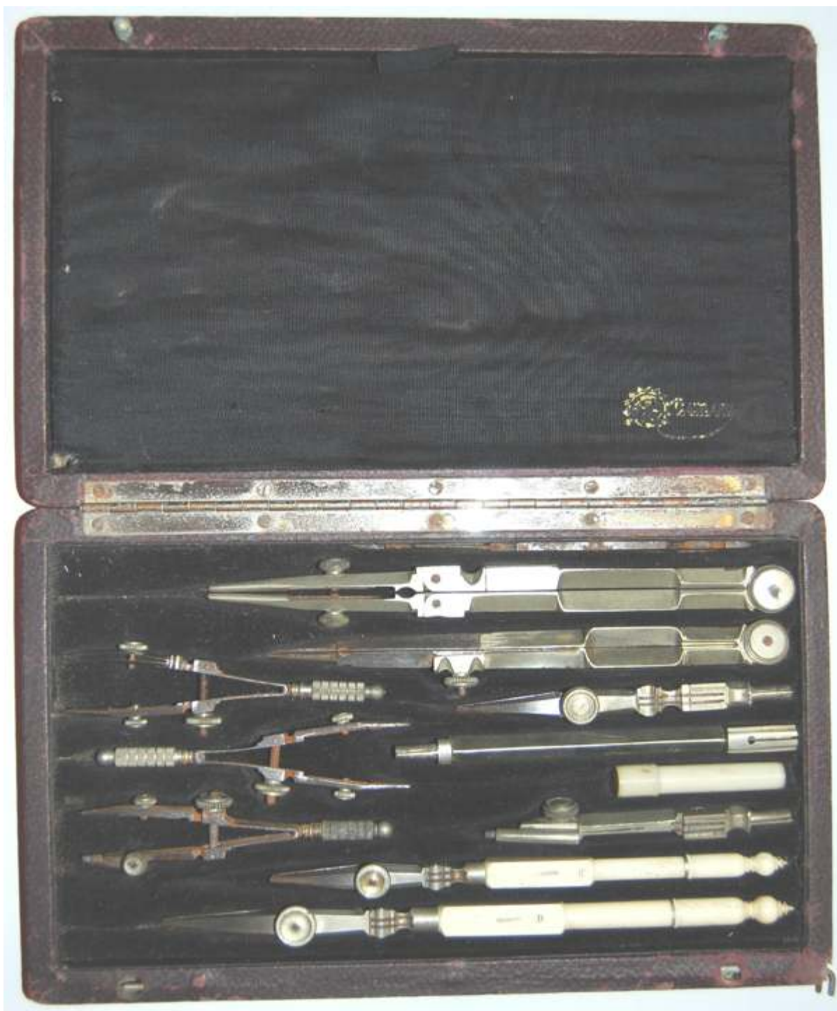
Fig. 306 Set of nickel silver instruments by Daimaru, Japan. The instruments include: a compass half set; hair dividers; three spring bows; two drawing pens; a knife key and a lead box. Although a copy of the English pattern the pens are unusual as the ends of the handle unscrew to reveal a pricker on the end of the main part of the handle.
