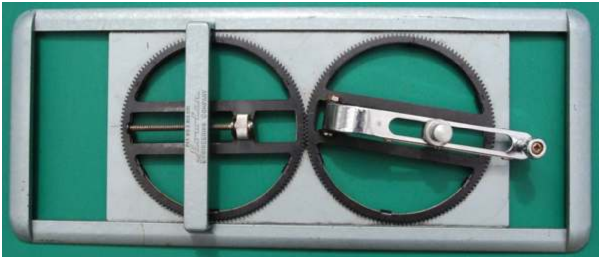
Fig. 152 Fowler ellipsograph model A-140
