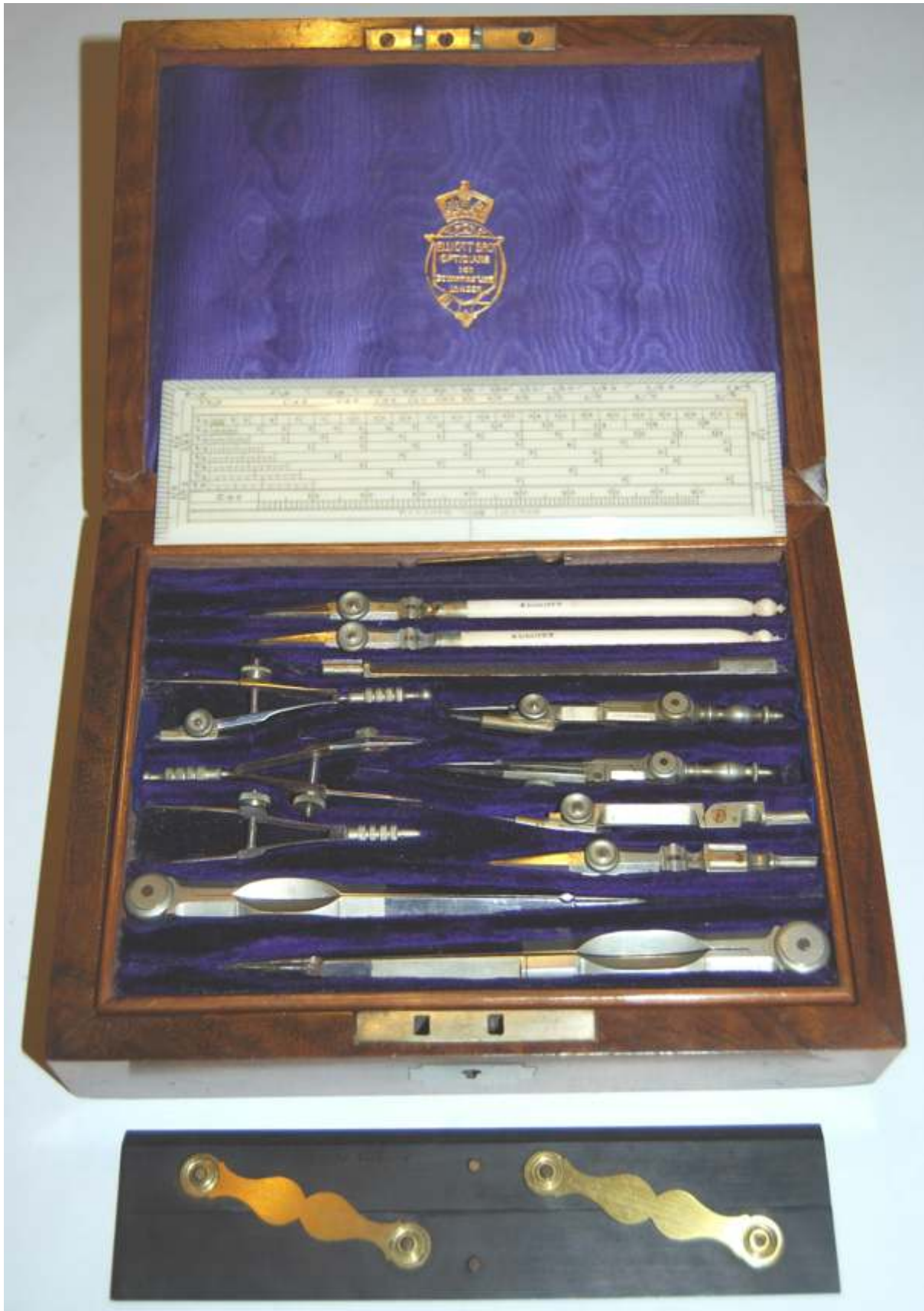
Fig. 304 A set of small size Elliott Brothers, 101 St. Martins Lane, London electrum instruments in a burr walnut veneered case. The ebony parallel rule and ivory protractor are both signed Elliott Bros., London. Late 19th century.
