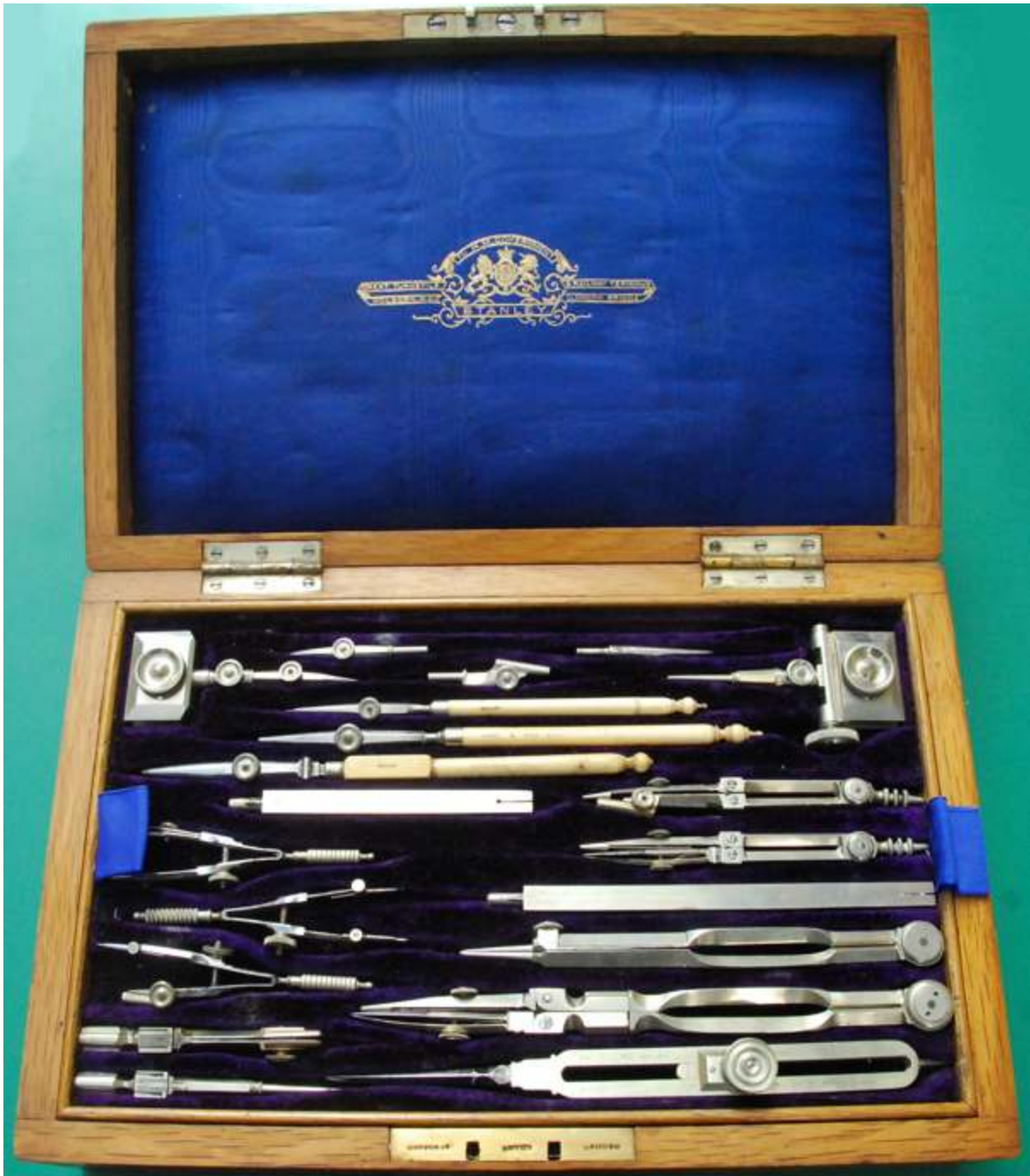
Fig, 298 W F Stanley ten inch electrum bound oak case of electrum drawing instruments, ca, 1880 The case has two lift out trays. The upper tray contains: a six inch compass with ink, pencil, type 'A' and type 'B' points and two lengthening bars; hair dividers; pen and pencil bow double jointed compasses; three spring bows; proportional divider; lifting nib and fine line ivory handled pens and an ivory handled pricker; Swiss pattern beam compass fittings. The lower tray contains an ivory sector, ivory rectangular protractor, and an ivory scale rule. The base of the box contains three vulcanite French curves.
