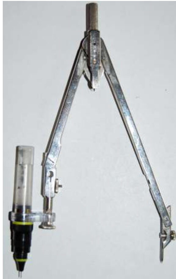
Fig. 237 Nestler compass with Rotring Variant pen unit attached.
