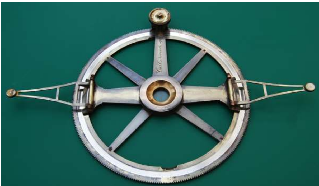
Fig. 42 Folding arm protractor by John Cail of Newcastle-upon-Tyne, probably 2nd quarter 19th century
