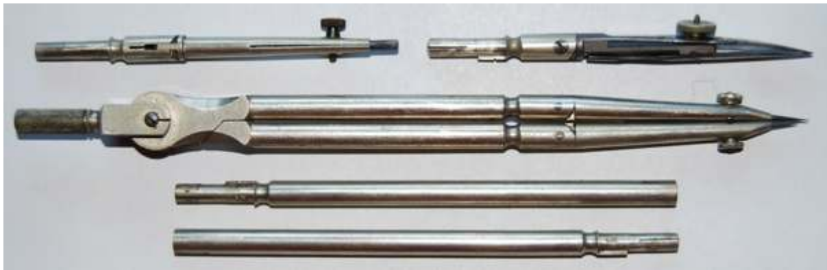
Fig. 196 Later type of Riefler round system compass dating from the 1930s
