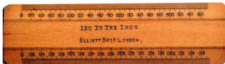
Fig. 67 Elliott Bros. 120 to the inch engine indicator scale
