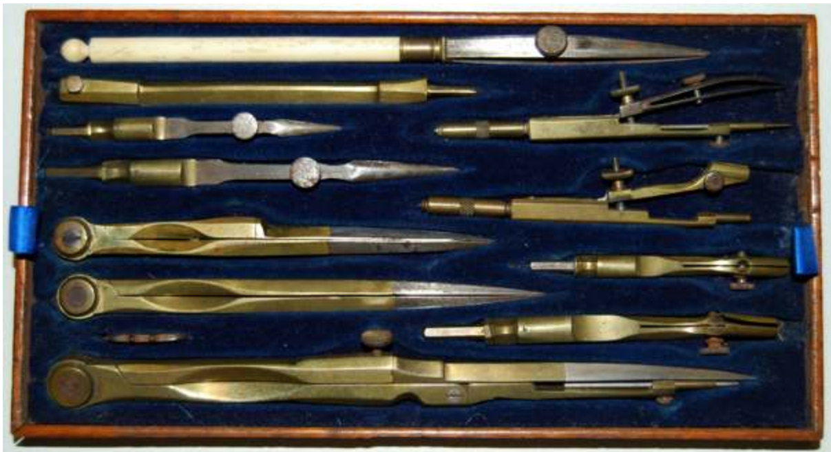
Fig. 165 Set of brass drawing instruments typical of those imported from France for student use.
