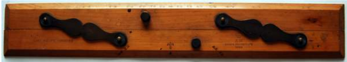
Fig. 71 Eighteen inch 'Capt. Field's Improved' parallel rule in boxwood & brass made in 1938 by Dargue Bros. for the Air Ministry
