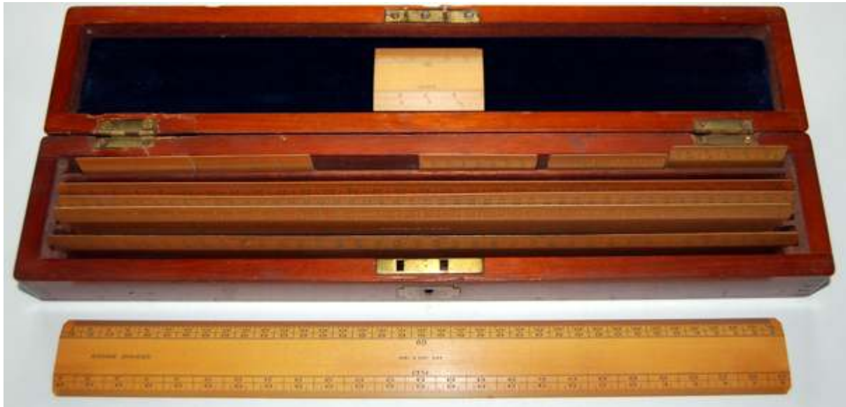
Fig. 63 Set of chain scales and offsets sold by the Army & Navy Cooperative Stores
